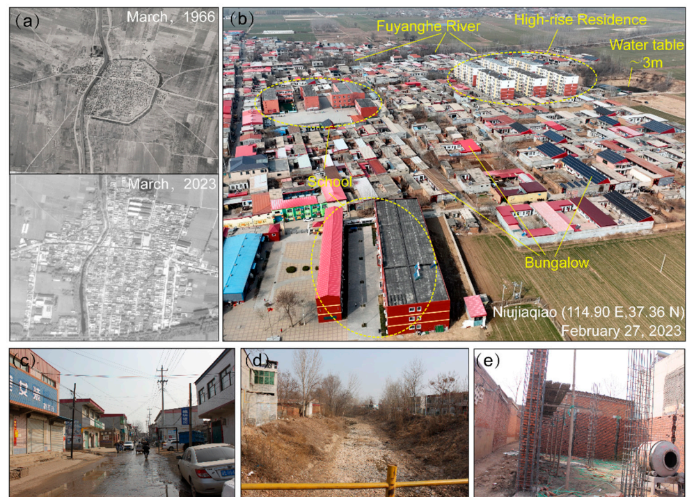
Figure 15. (a) Images of the range of buildings in Niujiqiao village in 1966 and 2023 at the locations shown in Figure 14; (b) UAV photo of Niujiqiao village near the epicenter of the earthquake on 8 March 1966 (taken on 27 February 2023), with most of the extended houses built as bungalows with no seismic-resistant measures and few of the school and residential buildings exhibiting seismic-resistant structures; (c) two-story houses next to streets with no seismic-resistant measures; (d) houses built around the adjacent dried-up river channel with no seismic-resistant structures; and (e) new construction of a small number of houses with structural columns.
