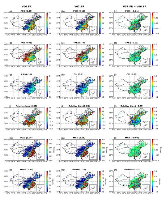
**Figure 10.** Spatial distribution of statistical metrics for IMERG V06 FR (**a**,**d**,**g**,**j**,**m**,**p**), IMERG V07 FR (**b**,**e**,**h**,**k**,**n**,**q**), and their differences (**c**,**f**,**i**,**l**,**o**,**r**) under extreme precipitation rate.
