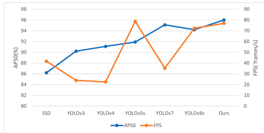
Figure 13. Line graph of FPS metrics and AP metrics for various algorithms. The blue line represents AP 50 , while the orange line indicates FPS.
