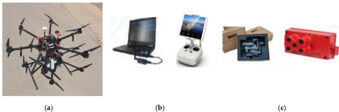
Figure 3. UAV multi-spectral image acquisition system: (a) unmanned aerial vehicle system; (b) flight control system; (c) holder and multi-spectral camera.
