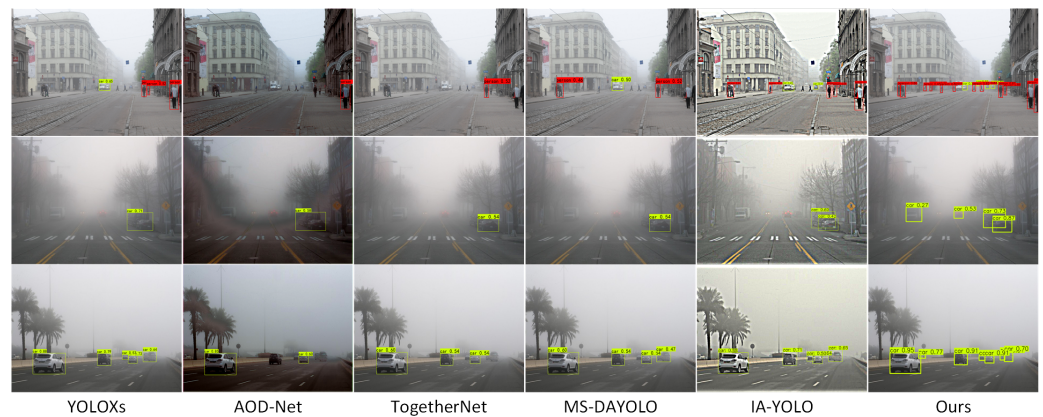
Figure 6. Detection results of our ODFC-YOLO and other advanced detection methods on Foggy Driving dataset. Obviously, the proposed ODFC-YOLO can detect more objects with higher confidence.
