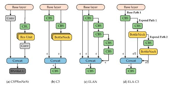
Figure 3. Evolution and exploration of the ELA-C3 module.
