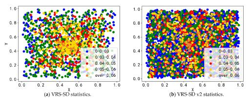
**Figure 9.** Distribution of target positions at different scales in VRS-SD and VRS-SD v2. The X and Y axes indicate the relative positions of the ships, and the image scale is normalized to a relative scale of  $1.0 \times 1.0$ . Different colors indicate the targets at different scales.
