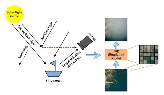
**Figure 1.** Fog simulation based on the optical model.
