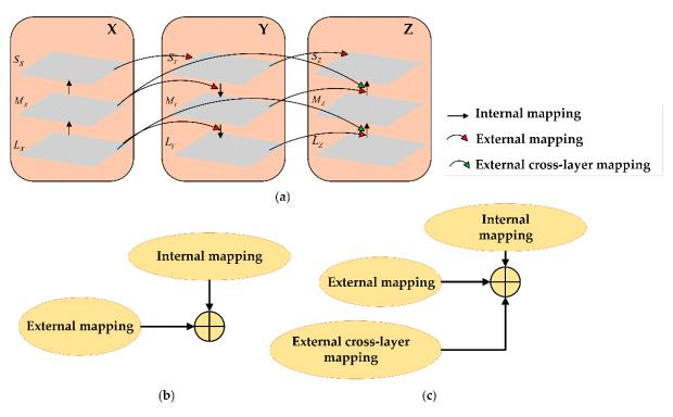
**Figure 5.** Abstract representation of fusion mapping. (a) Schematic diagram of a bidirectional fusion set. (b,c) Specific integration forms. The available features include the native feature set X, the top-down feature set Y, and the bottom-up feature set Z.
