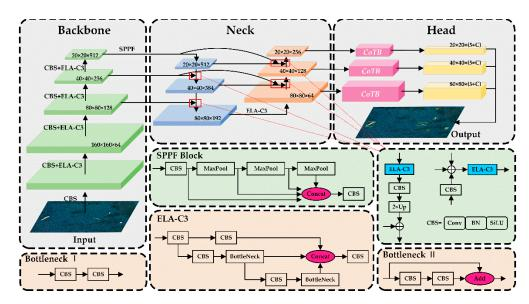
Figure 2. Overall architecture of the LMSD-Net framework.
