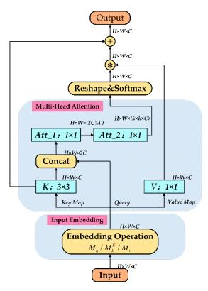
**Figure 7.** The detailed structures of the Contextual Transformer (CoT) block.  $\circledast$  denotes local matrix multiplication, and  $\oplus$  denotes the fusion of dynamic and static keys. For two consecutive  $1 \times 1$  convolutions, channel scaling factor  $\lambda$  is set as 4 in the experiment.
