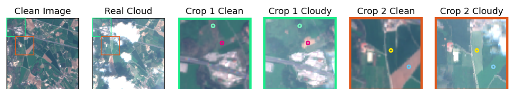
Figure 1. The approach of using pairs of real data for training and evaluating cloud removal models often results in fundamental differences in the ground surfaces. Examples from SEN12MS-CR [6]. It is apparent that some areas significantly change their state among acquisitions.
