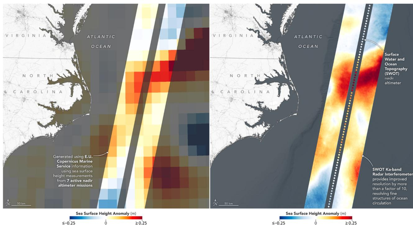
**Figure 2.** Comparison of the 25 km merged, multi-mission sea surface height anomaly (SSH-A) Level 4 data product from Copernicus Marine Environment Monitoring Service (CMEMS) with SWOT first light SSH-A imagery on 21 January 2023 shows the detection of structural features at about a 10-times-higher resolution for an area of the Gulf Stream off North Carolina. Image credit: NASA/JPL-Caltech, CNES, and CMEMS.
