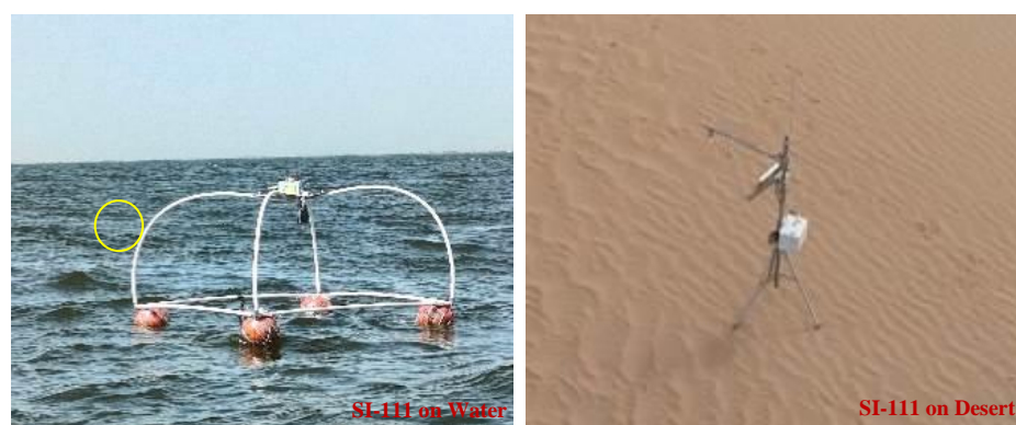
Figure 11. Part of the instrument layout diagram, including SI-111 on the waterbody ( left ) and SI-111 on the desert ( right ).
