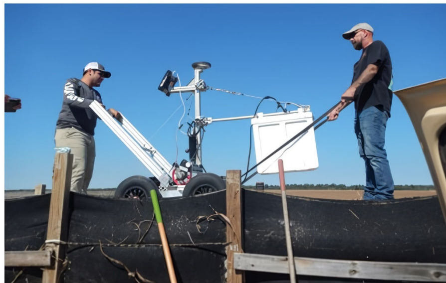
Figure 2. Photograph of data collection using IDS antenna array. Antenna was mounted on an aluminum cart and moved from one end of the trough to the other during data collection.
