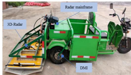
**Figure 9.** GPR data acquisition equipment.
