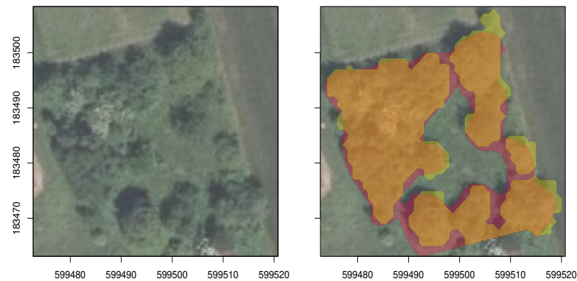
Figure 6. Vegetation polygon detected by the segmentation neural network (red polygon) merges narrow gaps and smooths vegetation edges in targets derived from LiDAR (yellow polygons). The scale is in meters, the CRS is EPSG:3794.
