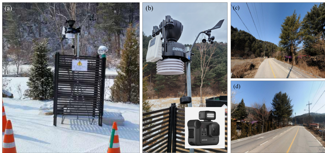
Figure 7. Meteorological observation station (a) and equipment composition (b) and its immediate surroundings in the (c) north and (d) south direction.
