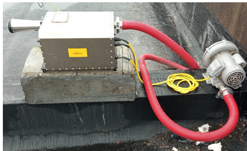
Figure 3. The actual installation of the FM-120 fog monitor.
