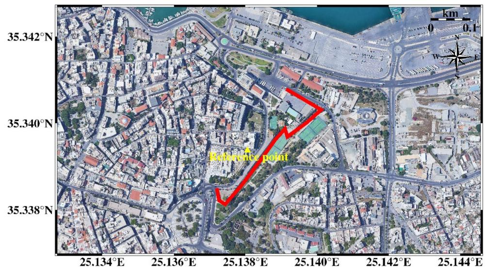
**Figure 4.** The location of the reference point marked by the yellow pin during D-InSAR and MSBAS processing of both ascending and descending SAR images. The background is Google Map. The red line represented the outline of the Sampionara Bastion.
