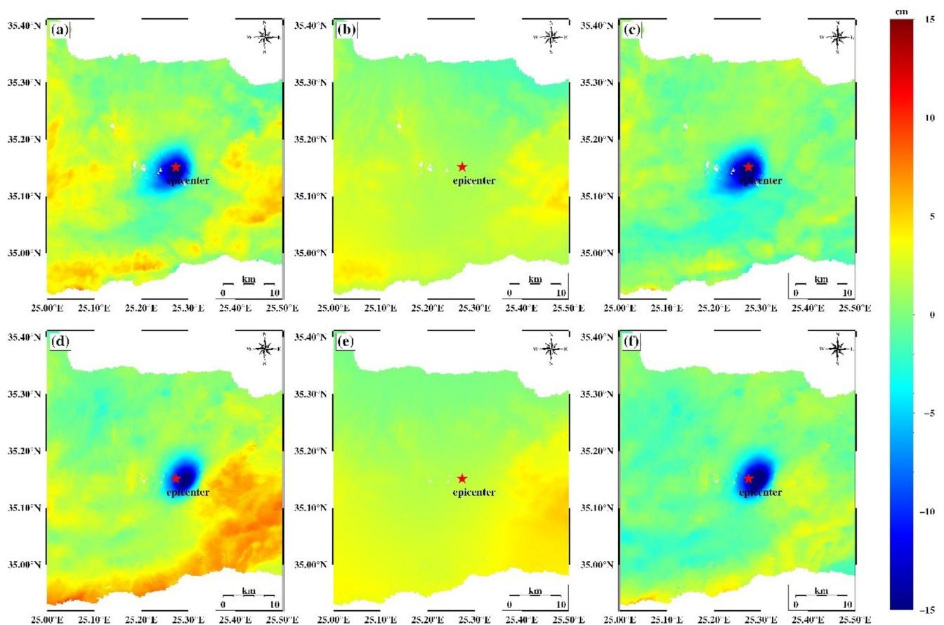
**Figure 5.** The GACOS corrections in D-InSAR processing. Positive value means uplift along the LOS direction. (a) Ascending uncorrected interferogram; (b) Tropospheric phase delay of the ascending interferogram calculated from GACOS; (c) GACOS corrected ascending interferogram; (d) Descending uncorrected interferogram; (e) Tropospheric phase delay of the descending interferogram calculated from GACOS; (f) GACOS corrected descending interferogram.
