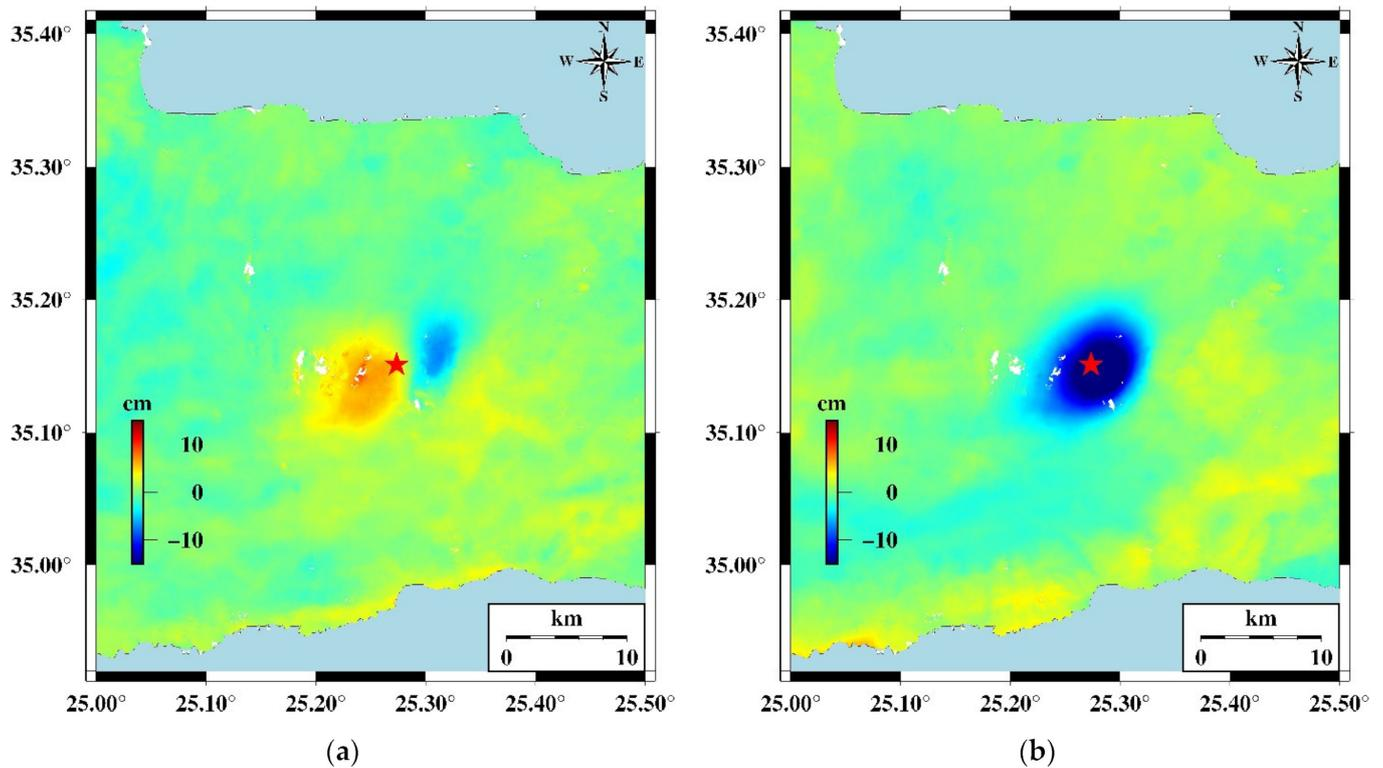
**Figure 6.** Two-dimensional co-seismic deformation field. The red star means the location of the epicenter. (a) EW deformation, positive to the east; (b) UD deformation, positive uplift.
