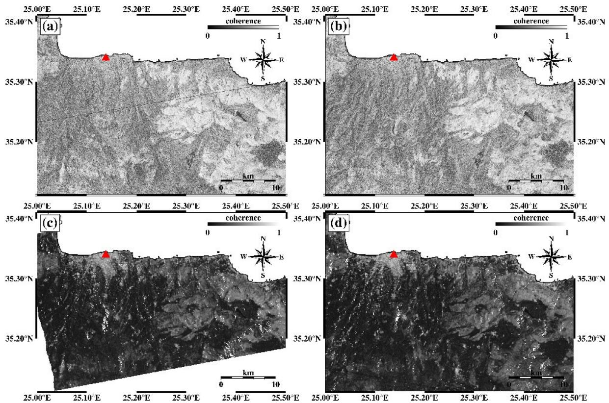
**Figure 3.** The selection of the reference point (Marked with red triangle). (a) Ascending D-InSAR coherence map; (b) descending D-InSAR coherence map; (c) ascending mean coherence calculated from a stack of 157 coherence maps; (d) descending mean coherence calculated from a stack of 152 coherence maps.
