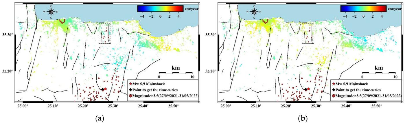
**Figure 8.** Two-dimensional deformation rate maps. The brown line represents the outline of the HCW. Black dash line marked the location of the 16–18 January, 2022, earthquake sequence larger than M 3.5 recorded by NOA-IG. Brown dots represent the earthquake events larger than M 3.5 during the entire observing period. Black solid lines represent the known faults referred to [7]. (a) EW deformation rates, positive to the east; (b) UD deformation rates, positive uplift.
