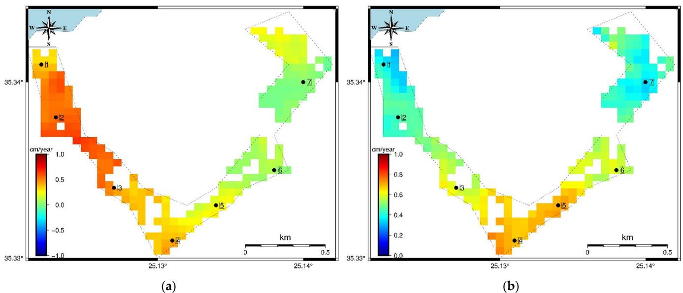
**Figure 9.** Two-dimensional deformation rates at the HCW site, the 7 black dots represent the 7 bastions as in Figure 2. (a) EW deformation rates, positive to the east; (b) UD deformation rates, positive uplift.
