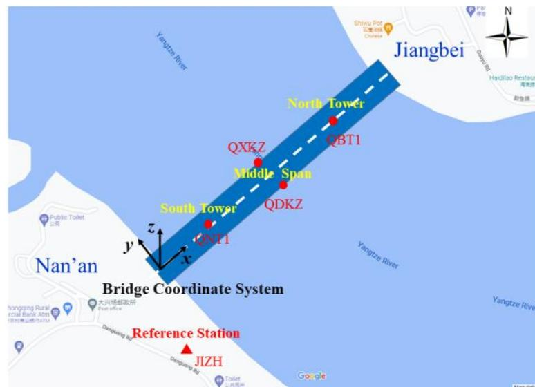
Figure 11. Low-cost GNSS stations are set up on the bridge. (The background figure is from Google Earth). The BCS is defined in this paper ( $x$  and  $y$  denote the longitudinal and lateral direction of the bridge and  $z$  is orthogonal with the plane of  $x$ - $o$ - $y$  and denotes the height direction).
