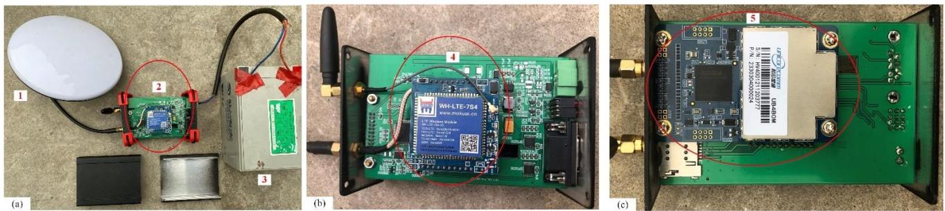
**Figure 7.** The prototypal low-cost GNSS sensor box and Micro PC mainboard. (a) The sensor box and Beitian BT-300 antenna. 1 = antenna, 2 = Micro PC mainboard, 3 = power supply; (b) The front of the Micro PC mainboard. 4 = WH-LTE-754 communication module; (c) The reverse side of the Micro PC mainboard. 5 = UB4BOM board with Nebulas-II UC4C0 system on chip (SoC).
