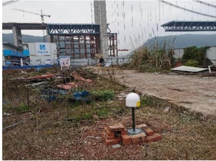
Figure 12. GNSS reference station JZHZ.
