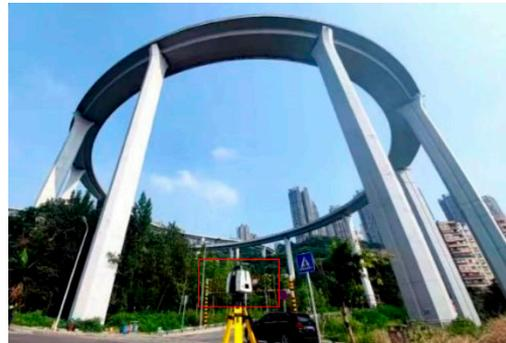
**Figure 6.** Sujiaba Bridge TLS data acquisition in scan station 1. The red box shows the Leica P50 3D laser scanner.
