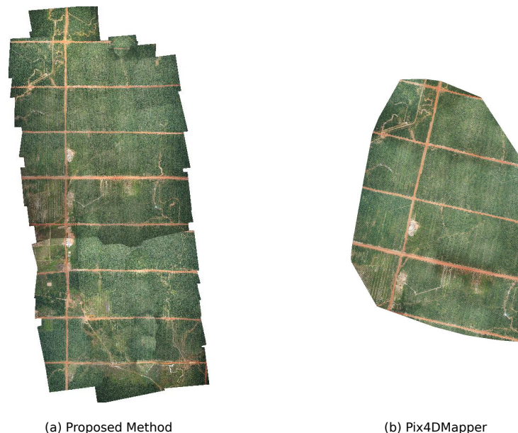
Figure 6. Images with low overlapping rate (30%) are collected for stitching comparison experiments between the proposed method (a) and Pix4DMapper (b).
