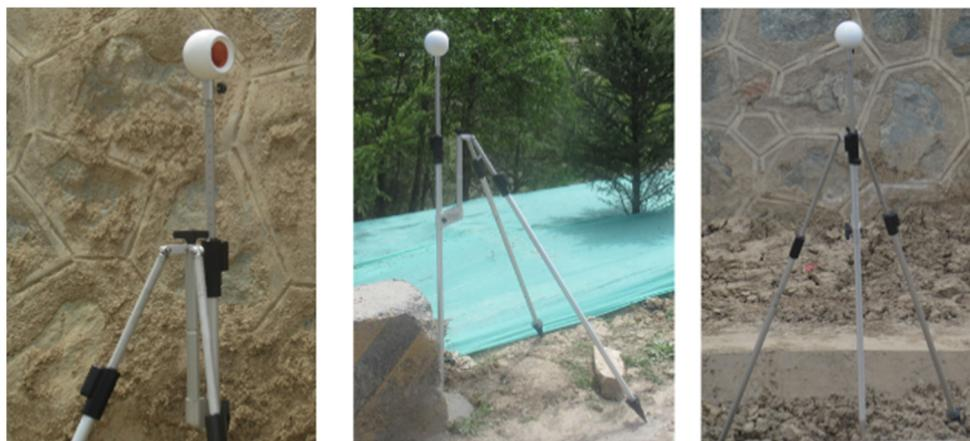
**Figure 10.** Prism ball target.
