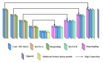
Figure 2. Structure diagram of L-Unet model; consists of downsampling, MFF module and upsampling.
