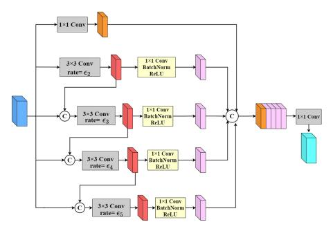
**Figure 4.** Multi-scale feature-fusion module based on dilated convolutions with different dilation rates.
