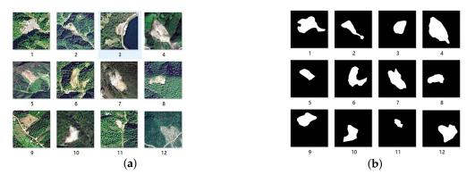
Figure 6. (a) Part of the landslide images for the test set and (b) extraction results of the L-Unet model.
