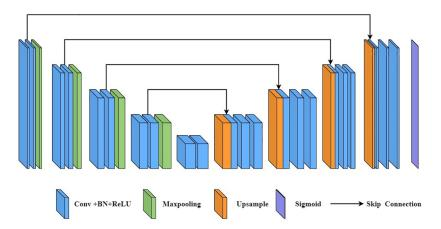
Figure 1. Structure diagram of U-Net model; consists of downsampling and upsampling.
