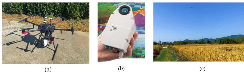
**Figure 2.** UAV image acquisition: (a) UAV platform, (b) Multispectral Rikola Camera, and (c) UAV flight experiments.
