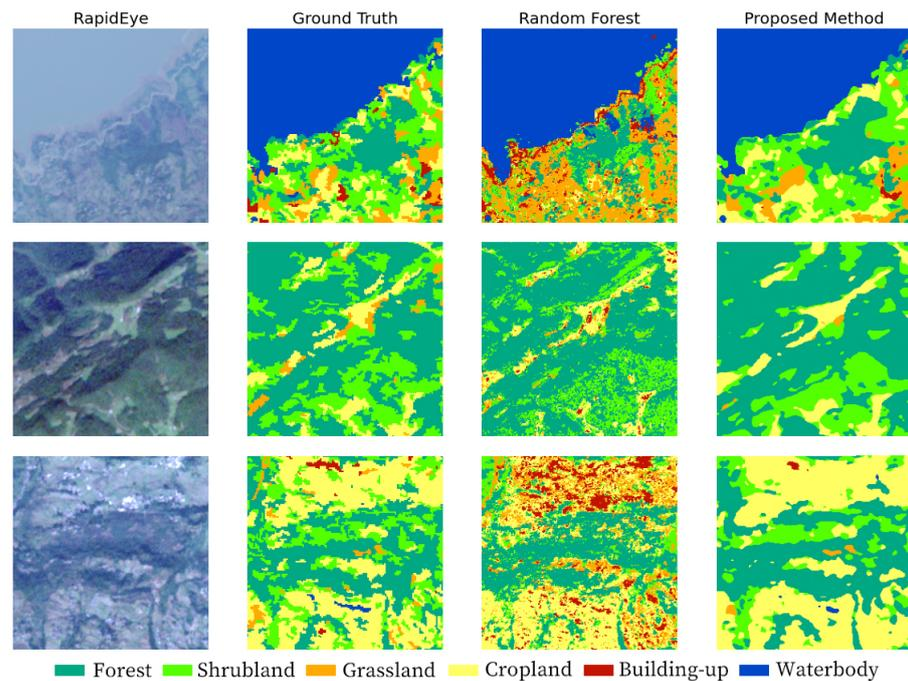
**Figure 11.** Comparison of random forest and proposed model outputs. The first column shows the RGB image, the second column shows the ground truth label, the third column shows the classification results from Random forest, and the fourth column shows the classification results from proposed model.
