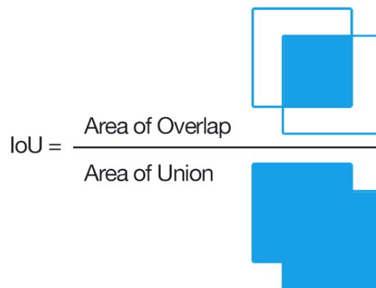
Figure 7. Illustration of IoU calculation. Source: Wikipedia.
