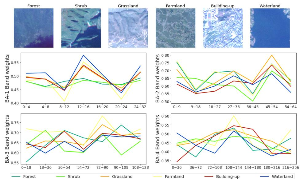
**Figure 14.** The band weights induced by the BA module at different depths in the proposed model. Six images from different categories were fed into the trained model and the weights for each band were class specific.
