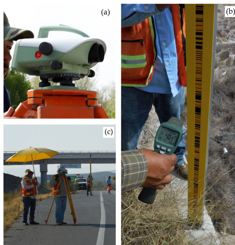
Figure 4. Equipment used by INEGI to perform the geodetic leveling surveys: (a) Leica DNA03 automatic digital level, (b) level rod with invar bar-code, and (c) benchmark leveling.
