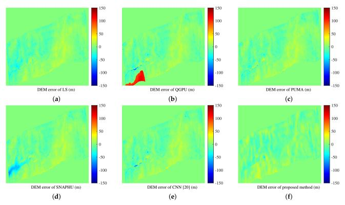
Figure 19. In the case of performing phase filtering, the DEM errors on real data. (a) DEM errors of the least squares method. (b) DEM errors of QGPU. (c) DEM errors of PUMA. (d) DEM errors of SNAPHU. (e) DEM errors of CNN [20]. (f) DEM errors of the proposed method.
