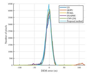
**Figure 20.** In the case of performing phase filtering, the fitted DEM error histogram curves of six phase unwrapping methods on real InSAR data.
