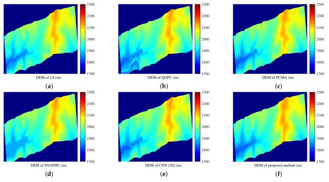
**Figure 18.** In the case of performing phase filtering, the DEM results of six phase unwrapping methods on real data. (a) LS. (b) QGPU. (c) PUMA. (d) SNAPHU. (e) CNN [20]. (f) Proposed method.
