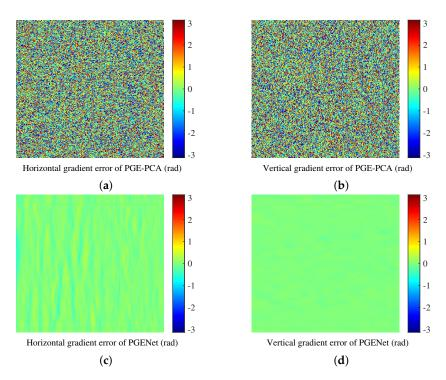
**Figure 10.** Phase gradient estimation errors. (**a**) Horizontal gradient error and (**b**) vertical gradient error of PGE-PCA. (**c**) Horizontal gradient error and (**d**) vertical gradient error of PGENet.
