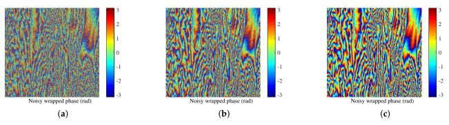
Figure 6. Examples of the noisy wrapped phase with different coherence coefficients. (a) 0.5. (b) 0.75. (c) 0.95.
