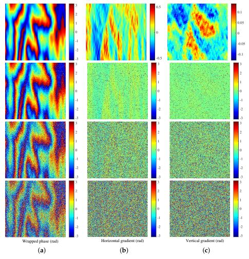
**Figure 2.** (a) Wrapped phase images, and (b,c) are the corresponding horizontal gradient images and vertical gradient images, respectively. From top to bottom, the coherence coefficients are 1, 0.95, 0.75, and 0.5, respectively.
