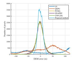
**Figure 23.** In the case of no phase filtering, the fitted DEM error histogram curves of six phase unwrapping methods on real InSAR data.
