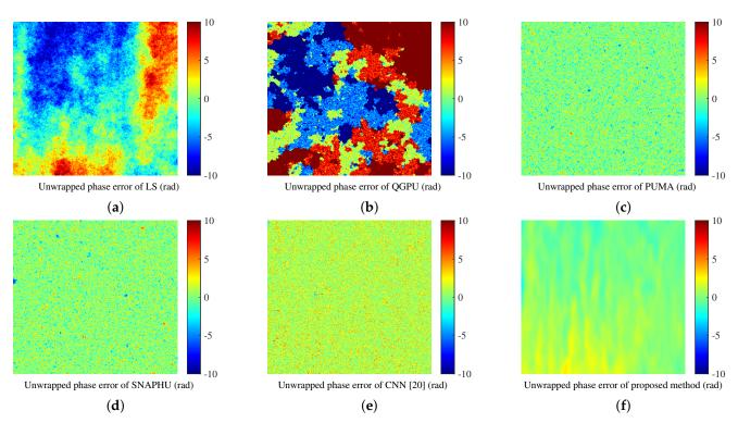
Figure 14. Unwrapped phase errors on simulated data. (a) LS. (b) QGPU. (c) PUMA. (d) SNAPHU. (e) CNN [20]. (f) Proposed method.
