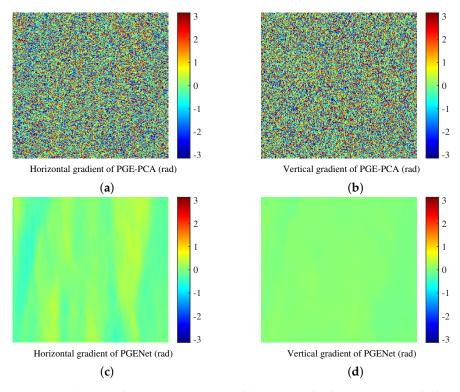
**Figure 9.** Phase gradient images estimated by two methods. (a) Horizontal phase gradient and (b) vertical phase gradient estimated by PGE-PCA. (c) Horizontal phase gradient and (d) vertical phase gradient estimated by PGENet.
