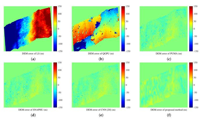
**Figure 22.** In the case of no phase filtering, the DEM errors on real data. (a) DEM errors of the least squares method. (b) DEM errors of QGPU. (c) DEM errors of PUMA. (d) DEM errors of SNAPHU. (e) DEM errors of CNN [20]. (f) DEM errors of the proposed method.
