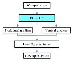
Figure 1. Flowchart of the traditional least squares phase unwrapping method.
