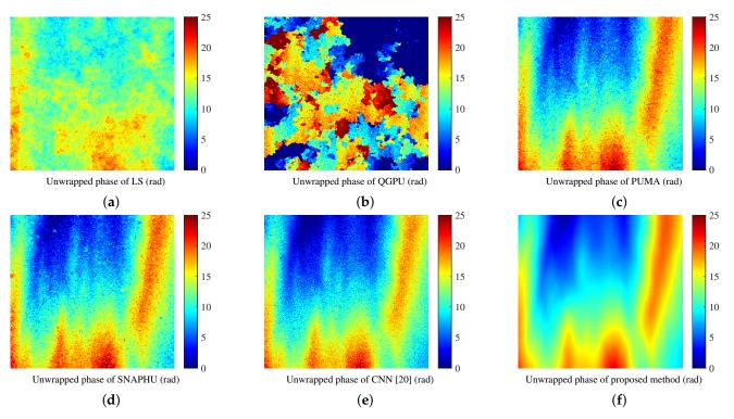
Figure 13. Unwrapped phase images of six phase unwrapping methods on simulated data. (a) LS. (b) QGPU. (c) PUMA. (d) SNAPHU. (e) CNN [20]. (f) Proposed method.
