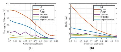
**Figure 16.** Quantitative indexes of six methods for phase unwrapping results on simulated wrapped phase images with different coherence coefficients. (**a**) Unwrapping failure rate. (**b**) Root mean square error (RMSE).
