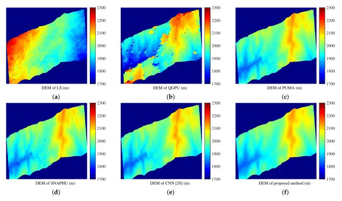
**Figure 21.** In the case of no phase filtering, the DEM results of six phase unwrapping methods on real data. (**a**) LS. (**b**) QGPU. (**c**) PUMA. (**d**) SNAPHU. (**e**) CNN [20]. (**f**) Proposed method.
