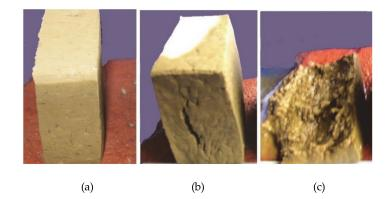
**Figure 4.** Liquefaction of a silty soil sample taken from the investigation site under the influence of moisture (sugar cube effect). (a) Dry soil sample, (b) soil sample after moistening, and (c) cross section of collapsed soil sample.
