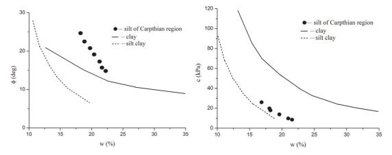
**Figure 9.** Internal friction angle ( $\Phi$ ) and cohesion (*c*) versus moisture content for tested silt samples collected from a depth of 0.5 to 5.5 m at the investigation site, presented on the background of other types of soils (own elaboration based on [31]).
