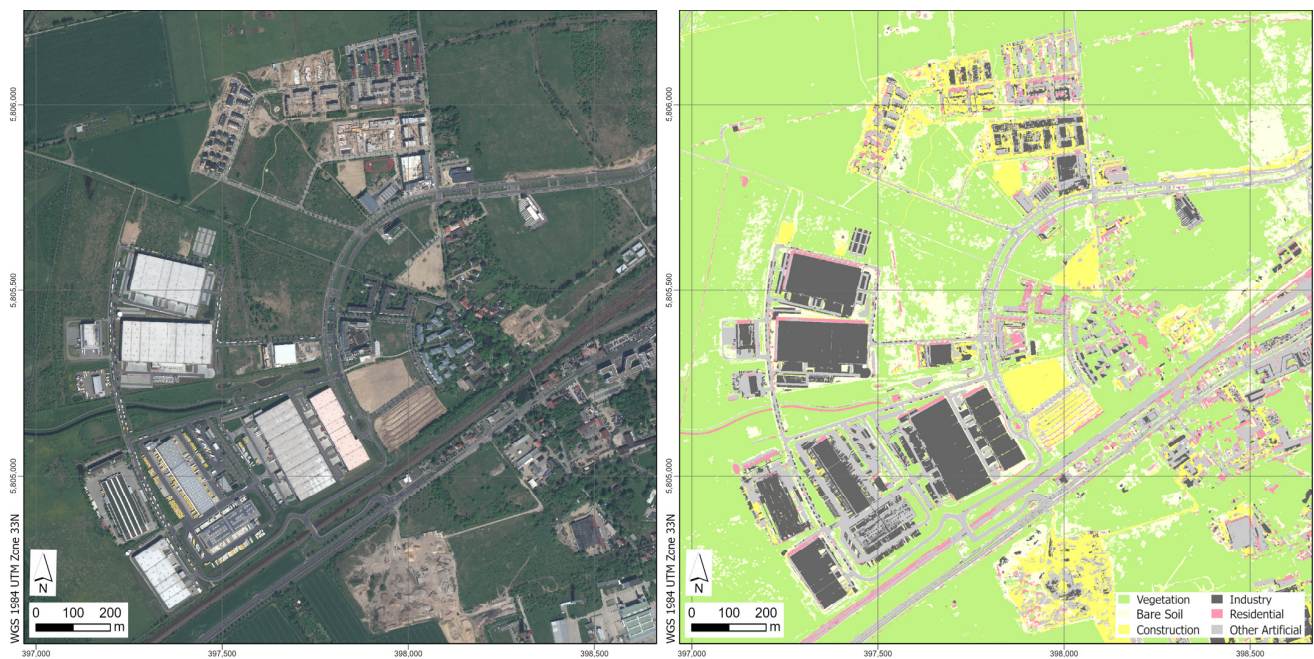
Figure 2. Detailed view of the classification results from the 29 April 2018. Source: WorldView Image ©2021, DigitalGlobe Inc., a Maxar company [22].
