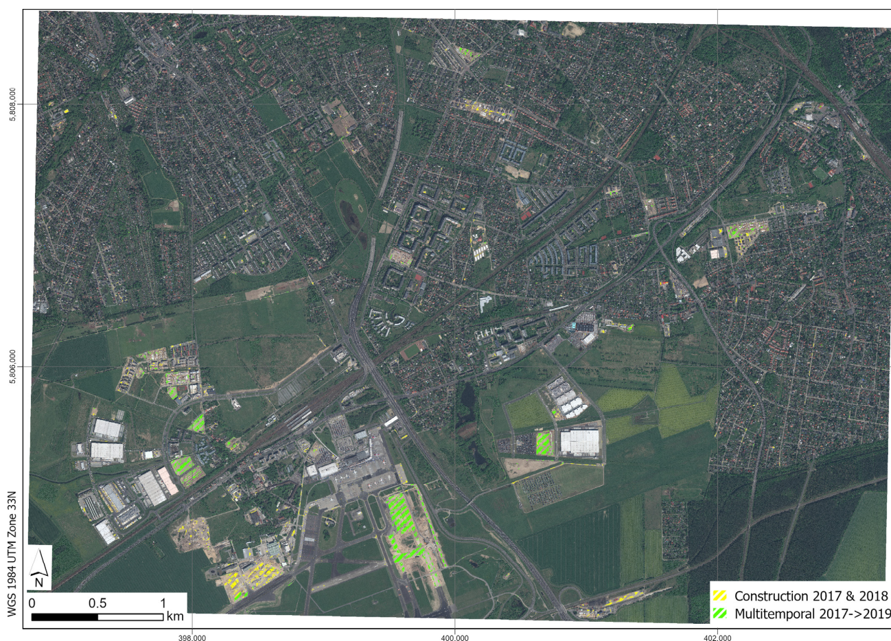
Figure 8. Combination of construction area detection in the full WorldView-3 scene of the 29 April 2018 using both multi-temporal approaches. Data source: WorldView Image ©2021, DigitalGlobe Inc., a Maxar company [22].
