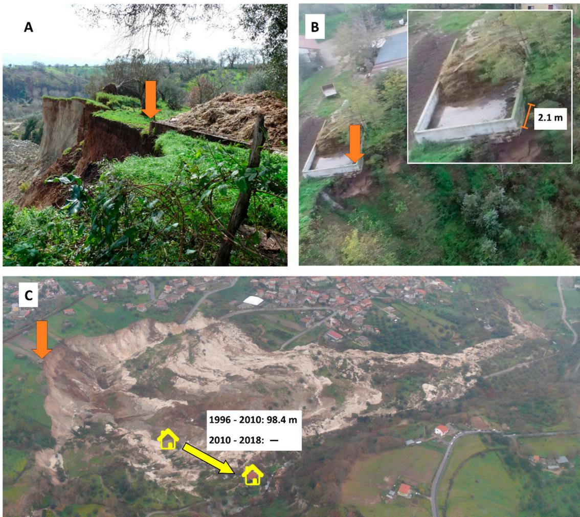
**Figure 12.** Evaluation of retrogressive evolution of the landslide: qualitative comparison between the terrestrial reconnaissance photograph (A) and the UAV survey (B); (C) measurement of the displacement of a building moved by the landslide.
