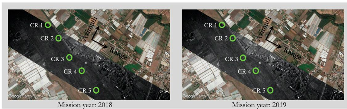
**Figure 1.** Multi-look amplitude SAR image (in geographic grid) patch of the entire acquired strip. The green circles indicate the CRs' positions. Left: relevant to the 2018 campaign. Right: relevant to the 2019 campaign.
