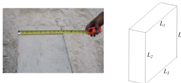
Figure 3. Measurement of dimensions (e.g., L_1 to L_4 ) of a structural element.
