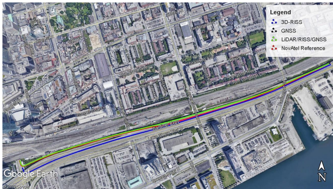
Figure 26. Navigation solution for 3D-RISS, GNSS, LiDAR/RISS/GNSS, and NovAtel reference at the Beginning of the Scenario.
