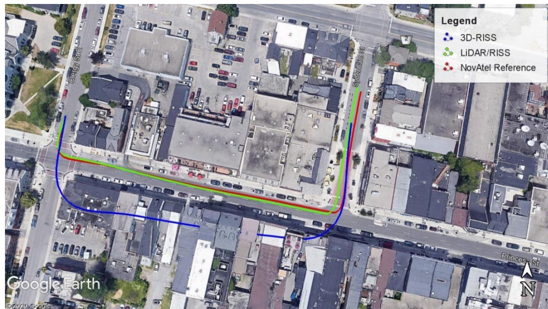
Figure 17. Navigation Solution for 3D-RISS, LiDAR/RISS, and NovAtel Reference during Simulated GNSS Outage 2, First Trajectory.
