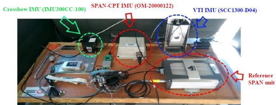
Figure 13. Sensor Setup on the Testbed.
