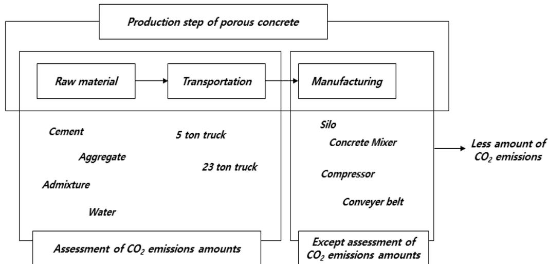
Figure 2. Porous vegetation concrete production stage and CO<sub>2</sub> emission analysis item.
