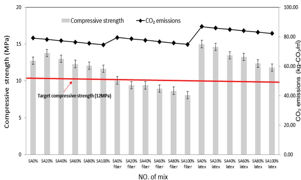
Figure 8. Relationship between amounts of CO<sub>2</sub> emission and compressive strength.
