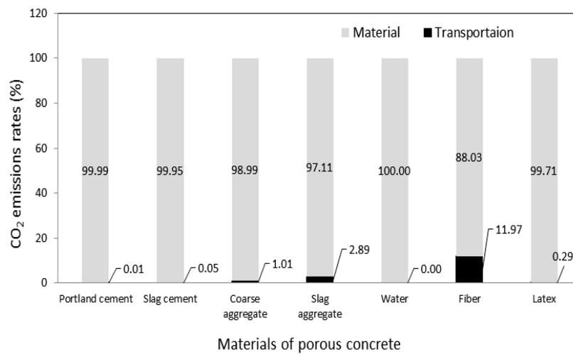
Figure 5. CO<sub>2</sub> emissions by production stage.
