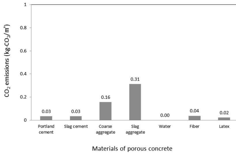
Figure 4. CO<sub>2</sub> emissions of transportation stage.
