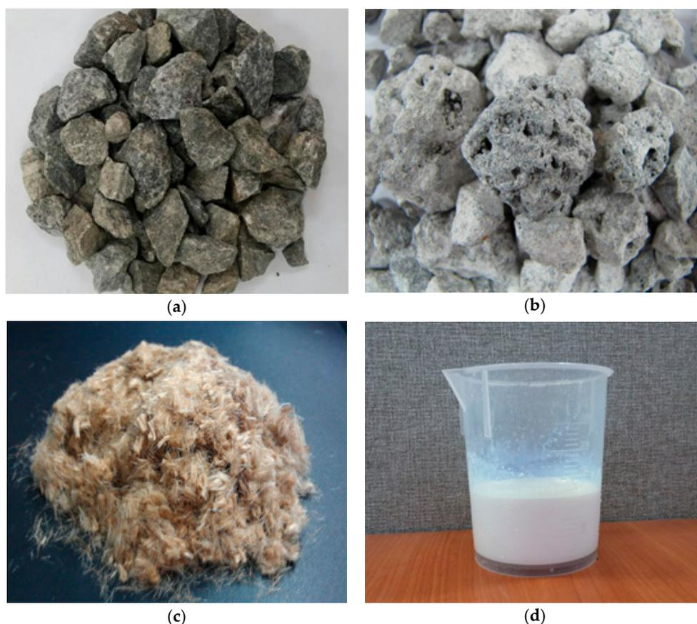
**Figure 1.** Materials. (a) Crushed aggregate; (b) Blast furnace slag aggregates; (c) Jute fiber; (d) Styrene butadiene (SB) latex.
