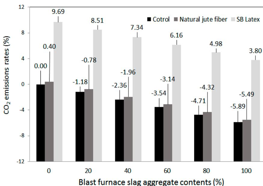
Figure 10. Increasing rate in CO<sub>2</sub> emissions from fiber reinforcement and latex use.
