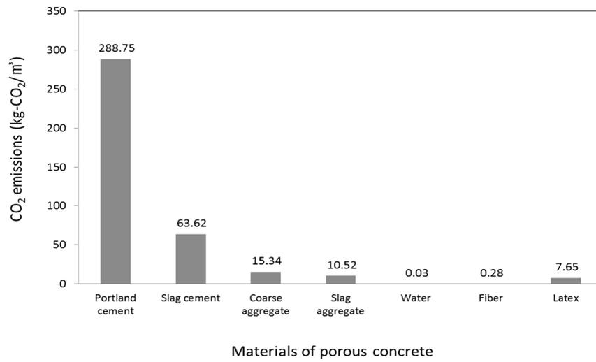
Figure 3. CO<sub>2</sub> emissions of materials stage.
