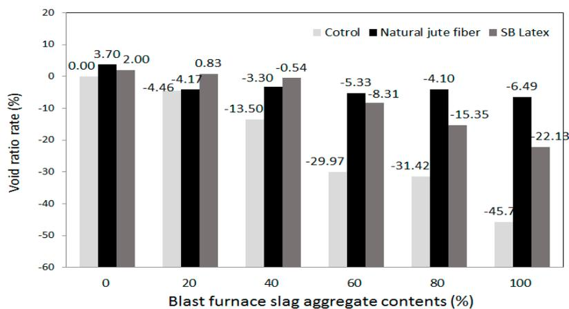
Figure 7. Void ratio increasing rate according to blast furnace slag replacement rate.
