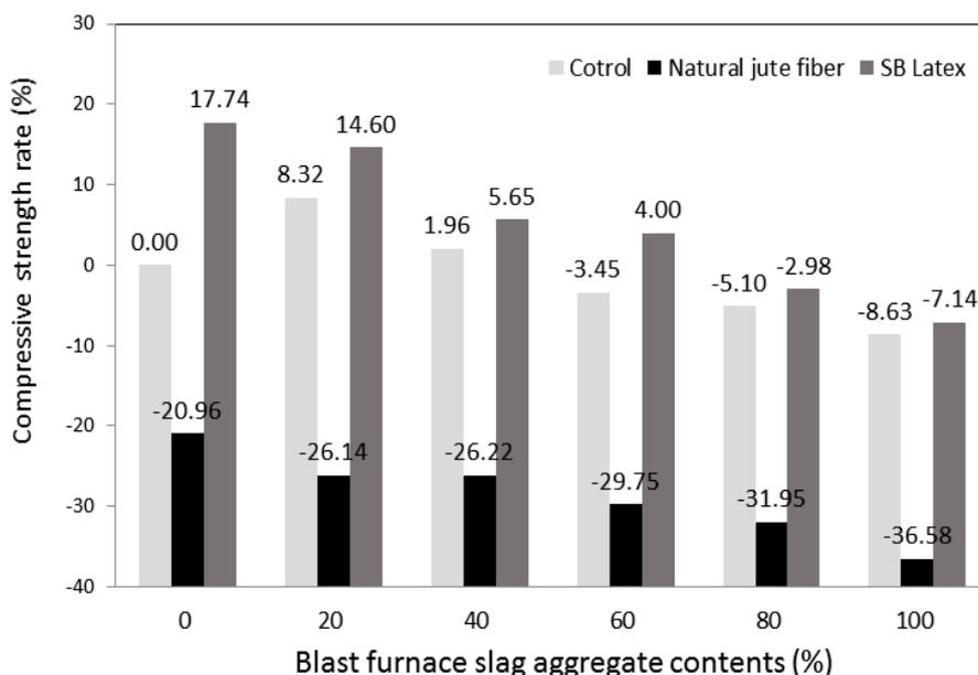
Figure 9. Increase rate in compressive strength according to use of fiber reinforcement and latex.
