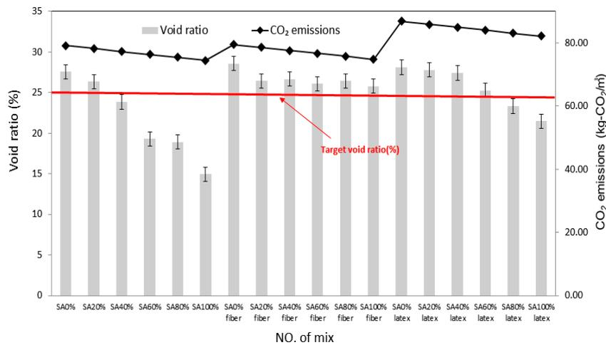
Figure 6. Analysis of void ratio and CO<sub>2</sub> reduction effect.
