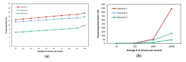
**Figure 6.** Performance comparison based on three scenarios: (**a**) Processing time given the average number (#) of sensors data sent to the server per second from 10 until 100 sensors data; (**b**) Processing time given the average number of sensors data sent to the server per second from 10 until 10,000 sensors data.
