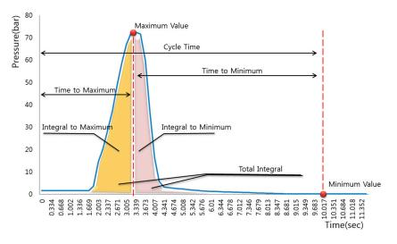
Figure 5. One set of features variable from injection pressure data.
