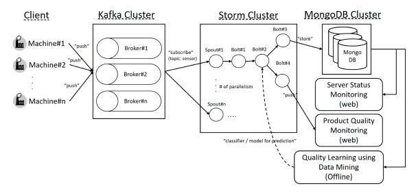
Figure 1. Open source-based real-time data processing (OSRDP) architecture framework.
