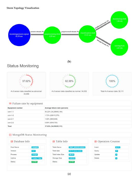
**Figure 2.** The web-based monitoring pages: (**a**) real-time quality monitoring; (**b**) Apache Storm topology status monitoring; (**c**) Server status monitoring.
