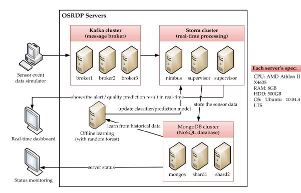
Figure 4. Configuration for simulation test.
