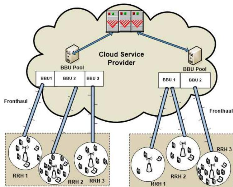
**Figure 1.** Fifth-generation (5G) Cloud Radio Access Network (CRAN) service architecture. BBU: baseband processing unit; RRH: remote radio head.
