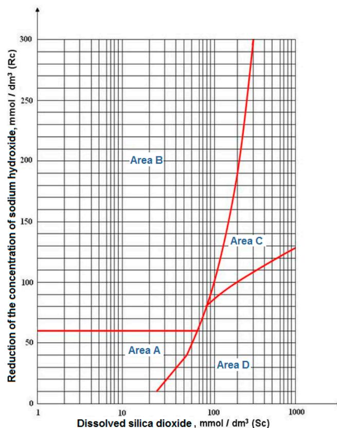
**Figure 3.** Verification of the reaction alkali–gregates: aggregates from zone A are non-reactive and are recommended for utilization; aggregates from zone B are generally unreactive; aggregates from zone C are characterized by a potentially significant reactivity; and aggregates from zone D are considered harmful.
