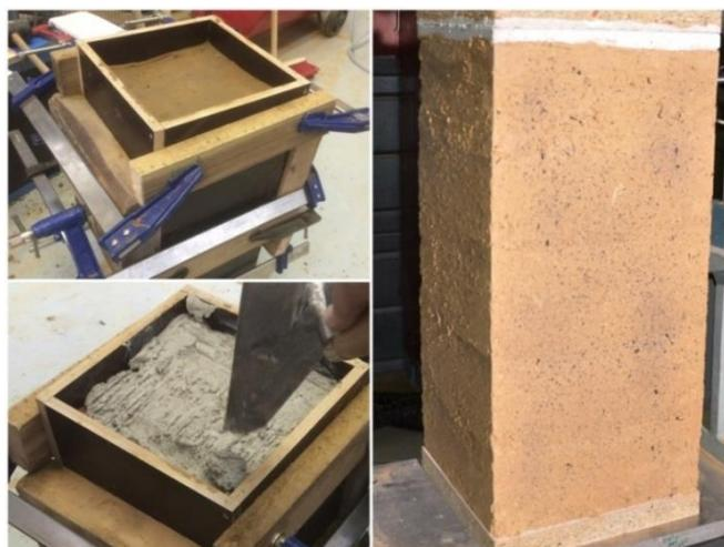
**Figure 6.** Prismatic specimen manufactured from Soil A, surfaced with a lime mortar.
