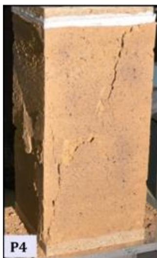
Figure 9. A specimen after the uniaxial compression test.
