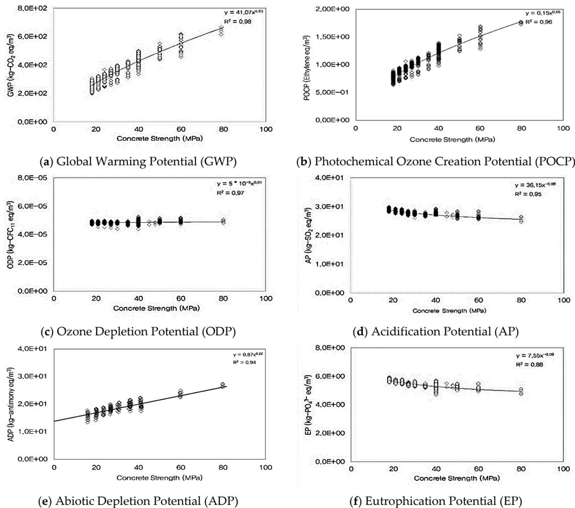
**Figure 4.** Environmental impact analysis by concrete strength.
