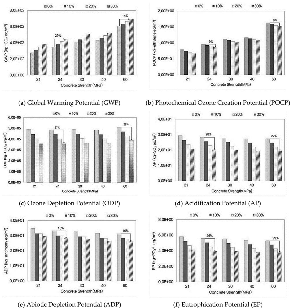
Figure 6. Environmental impact analysis by recycled aggregate mixing ratio.
