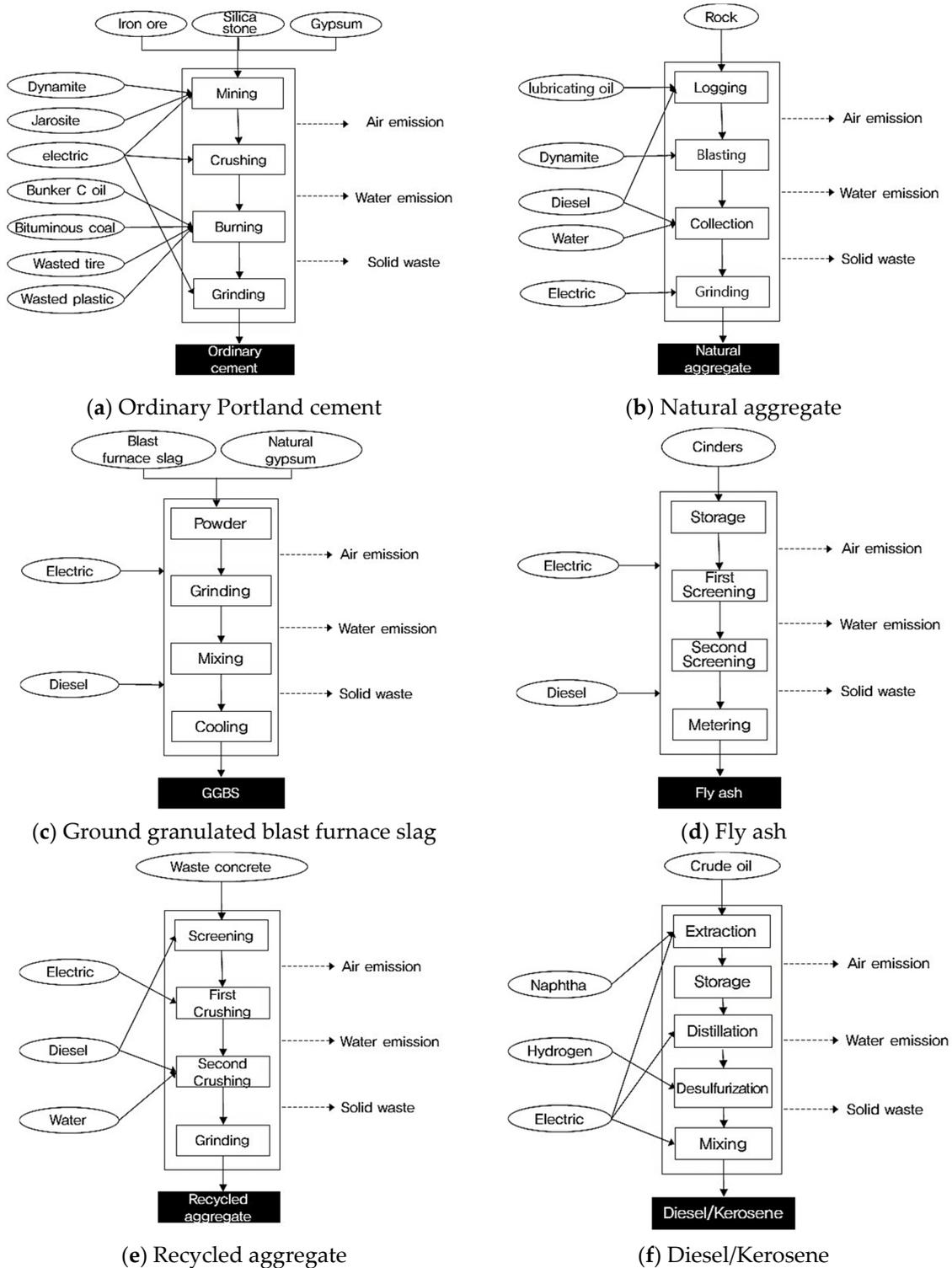
Figure 3. Production process of raw material and oil.
