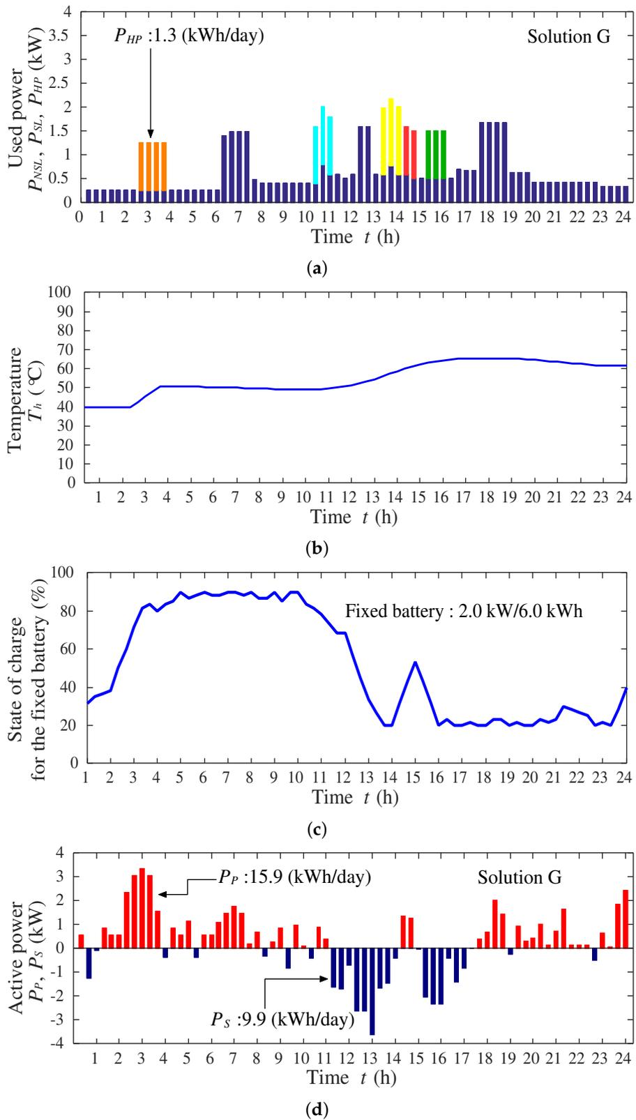
**Figure 18.** Simulation result for Solution G (Case 3): (a) used power of the appliances and the HP; (b) water temperature in the storage tank; (c) state of charge for the fixed battery; (d) purchased and sold power.
