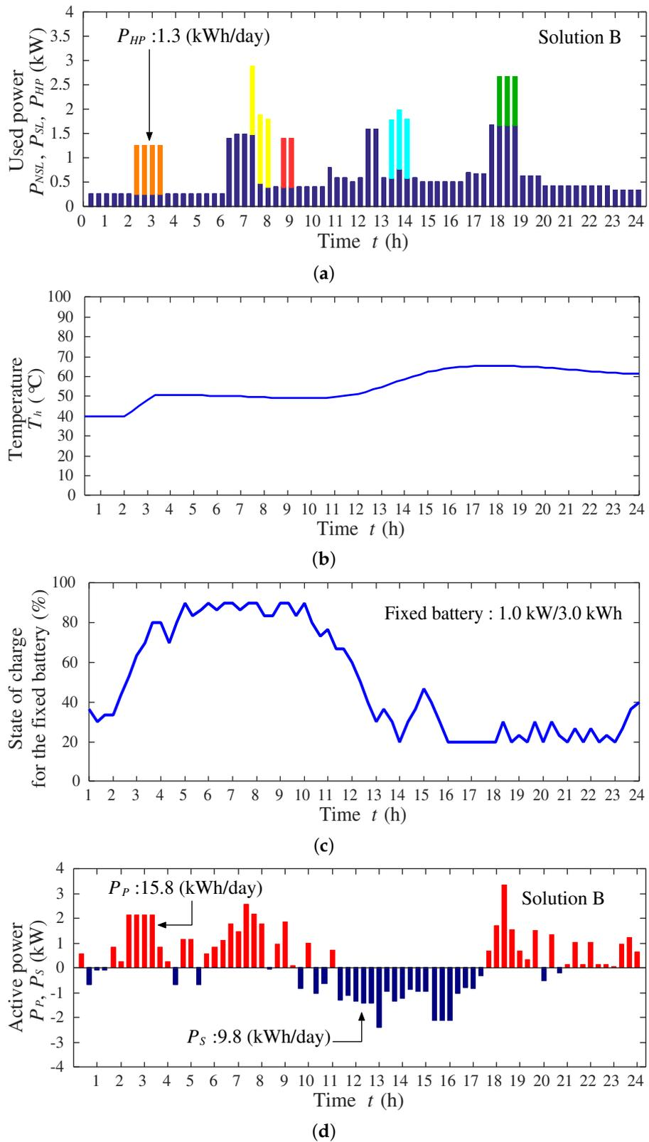
**Figure 13.** Simulation result for Solution B (Case 1): (a) used power of the appliances and the HP; (b) water temperature in the storage tank; (c) state of charge for the fixed battery; (d) purchased and sold power.
