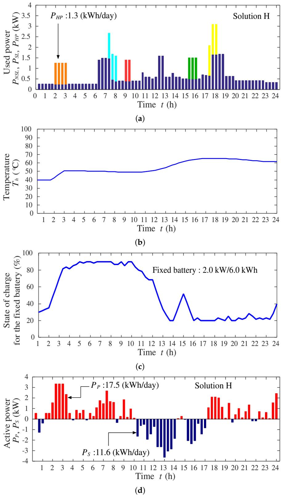
**Figure 19.** Simulation result for Solution H (Case 3): (a) used power of the appliances and the HP; (b) water temperature in the storage tank; (c) state of charge for the fixed battery; (d) purchased and sold power.
