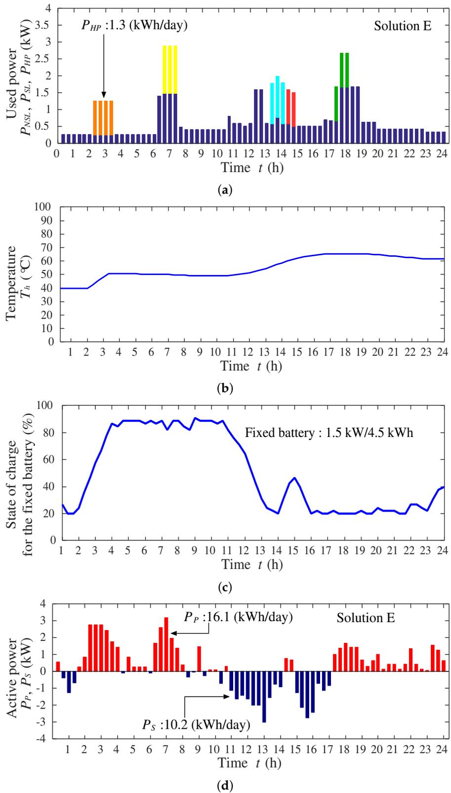
**Figure 16.** Simulation result for Solution E (Case 2): (a) used power of the appliances and the HP; (b) water temperature in the storage tank; (c) state of charge for the fixed battery; (d) purchased and sold power.
