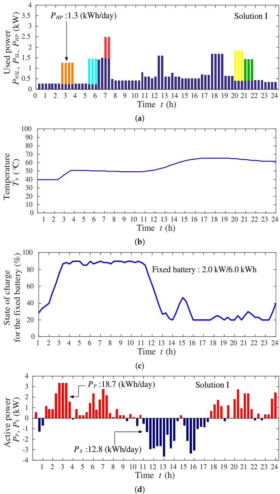
**Figure 20.** Simulation result for Solution I (Case 3): (a) used power of the appliances and the HP; (b) water temperature in the storage tank; (c) state of charge for the fixed battery; (d) purchased and sold power.
