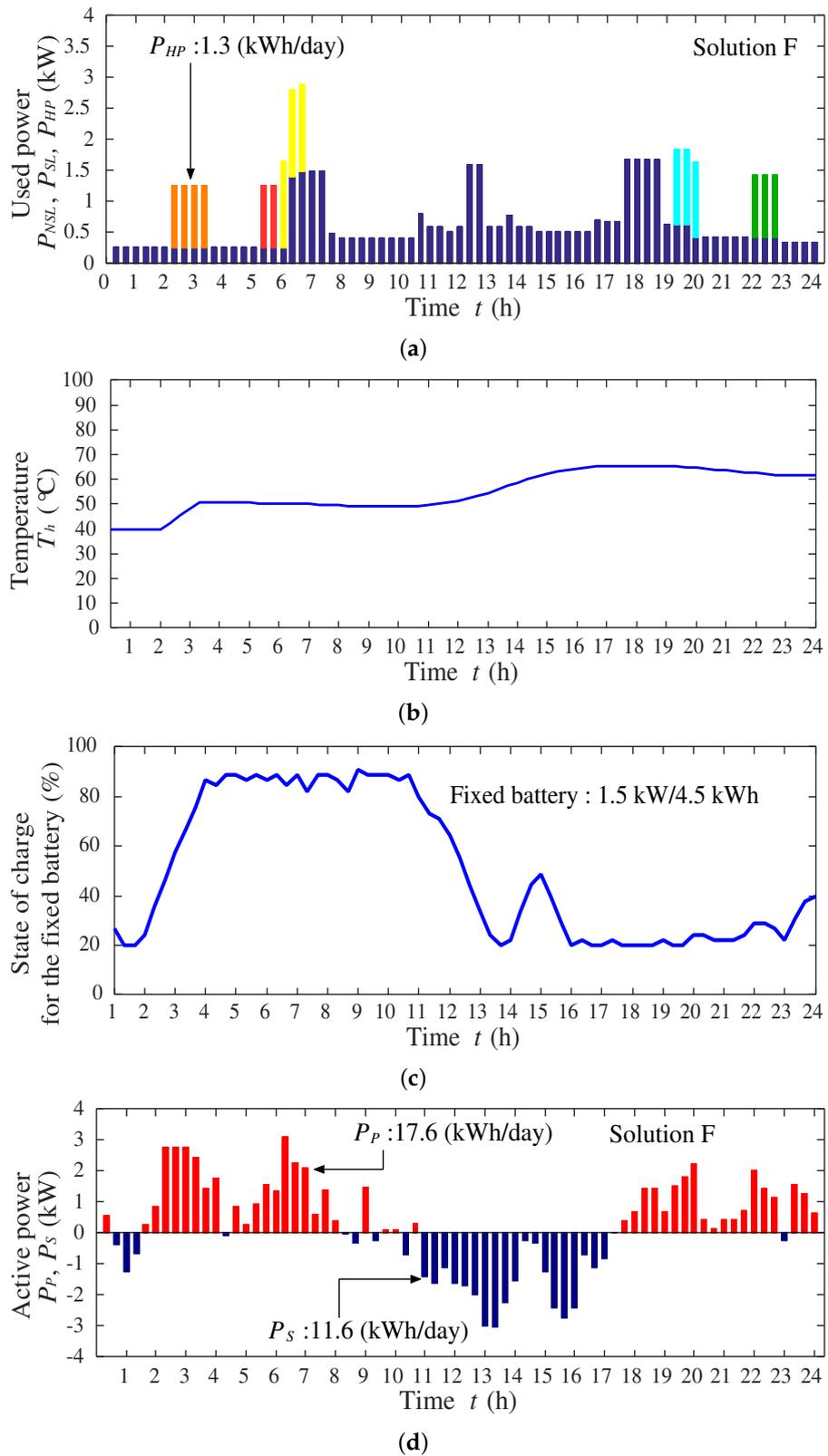
**Figure 17.** Simulation result for Solution F (Case 2): (a) used power of the appliances and the HP; (b) water temperature in the storage tank; (c) state of charge for the fixed battery; (d) purchased and sold power.
