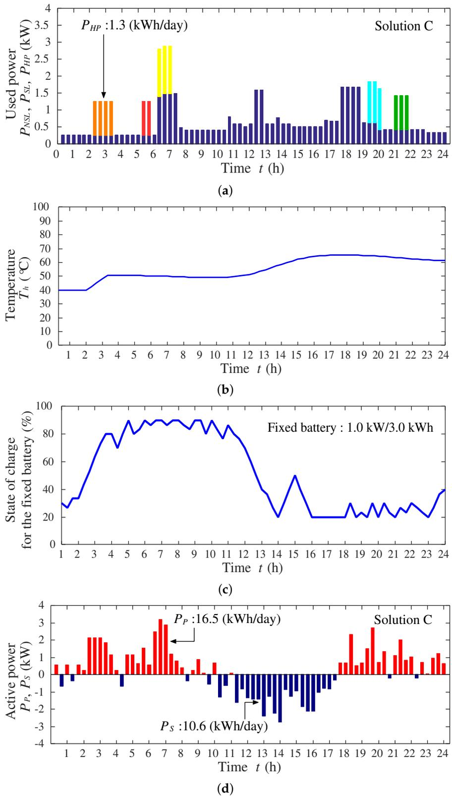
**Figure 14.** Simulation result for Solution C (Case 1): (a) used power of the appliances and the HP; (b) water temperature in the storage tank; (c) state of charge for the fixed battery; (d) purchased and sold power.
