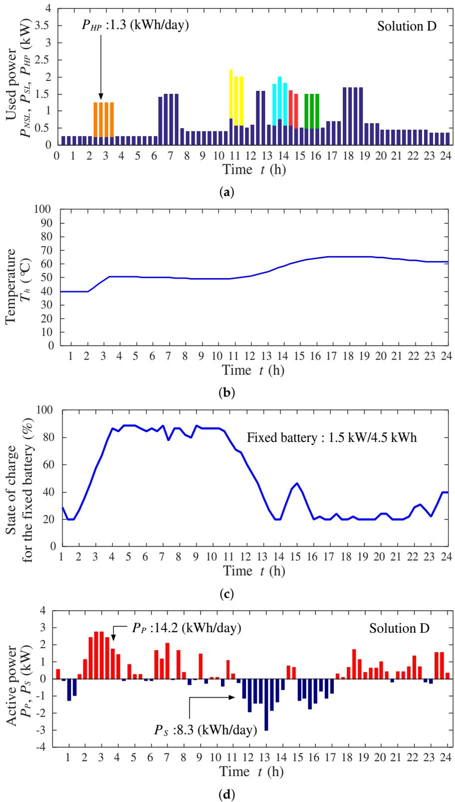
**Figure 15.** Simulation result for Solution D (Case 2): (a) used power of the appliances and the HP; (b) water temperature in the storage tank; (c) state of charge for the fixed battery; (d) purchased and sold power.
