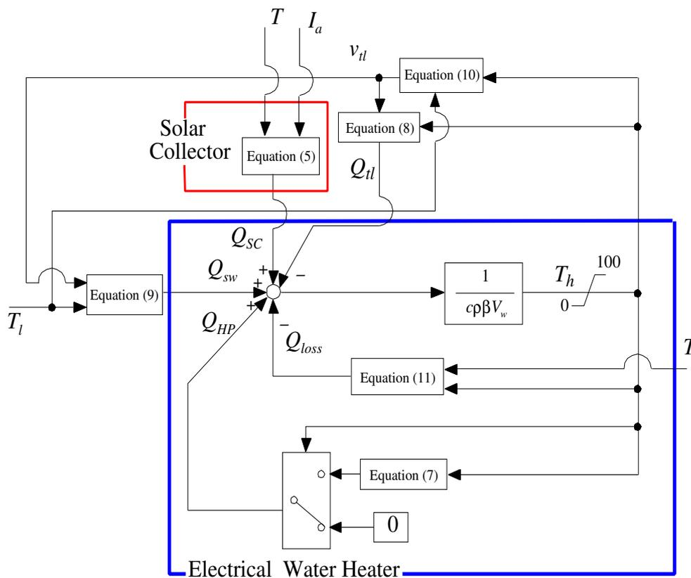
Figure 4. Model of the solar collector system.
