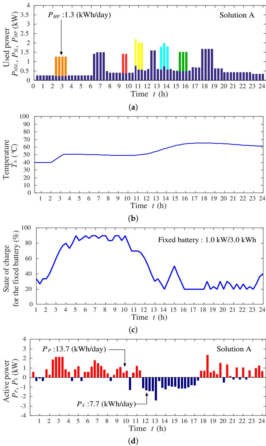
**Figure 12.** Simulation result for Solution A (Case 1): (a) used power of the appliances and the Heat Pump (HP); (b) water temperature in the storage tank; (c) state of charge for the fixed battery; (d) purchased and sold power.
