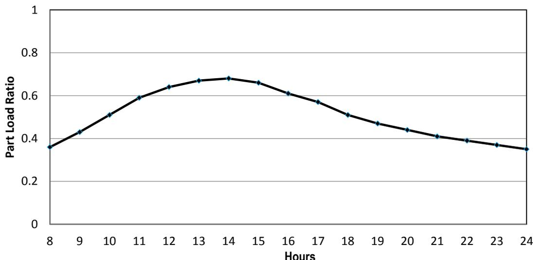
**Figure 15.** Seasonal average part load ratio of air conditioning system during the operation period.
