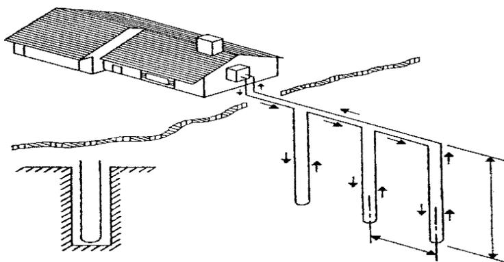
**Figure 2.** Vertical U-bend series flow.
