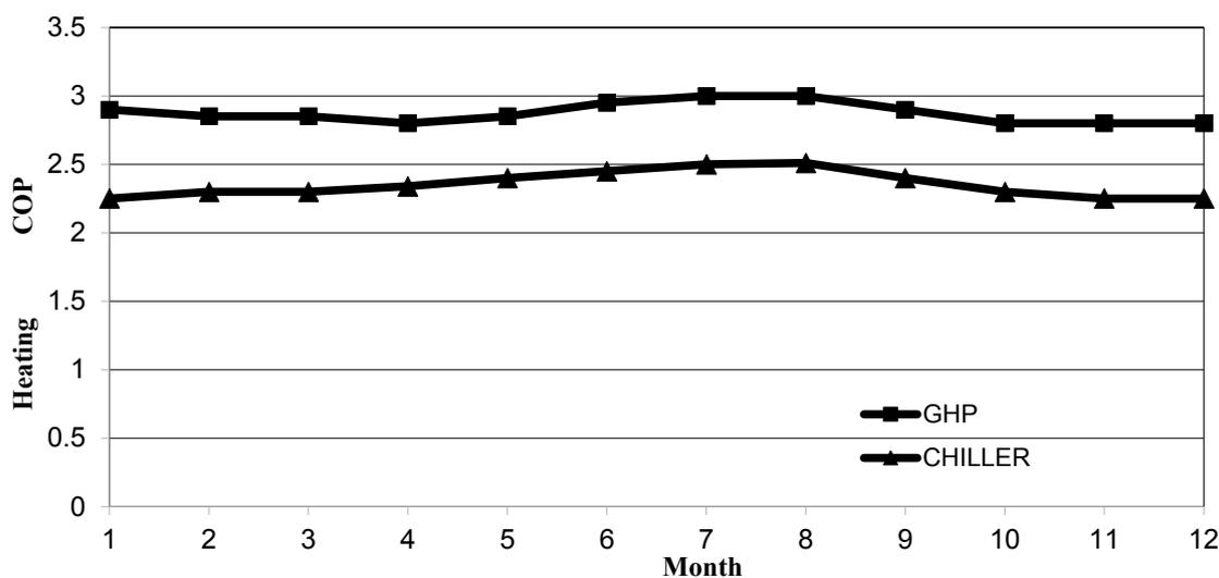
**Figure 14.** Monthly heating COPs for the geothermal heat pump and air-cooled heat pump chiller systems.
