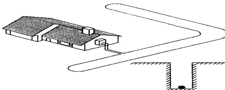
**Figure 1.** Single-layer horizontal ground loop.
