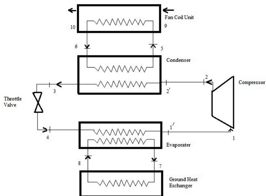
**Figure 4.** Schematic diagram of an air conditioning system for winter operations.
