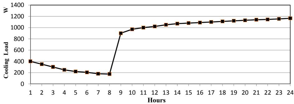
Figure 10. Hourly cooling load for light.
