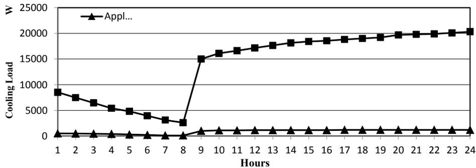
Figure 11. Hourly cooling load for equipment.
