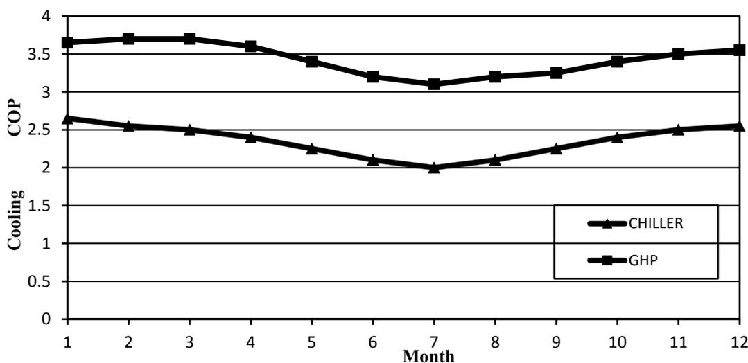
**Figure 13.** Monthly cooling COPs for the geothermal heat pump and air-cooled heat pump chiller systems.
