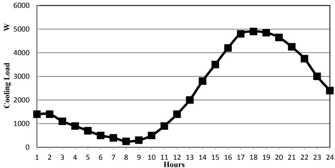
Figure 6. Hourly cooling load for roof.
