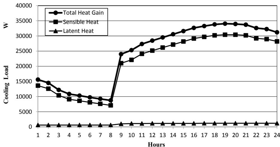
Figure 12. Hourly cooling load for total heat gain.
