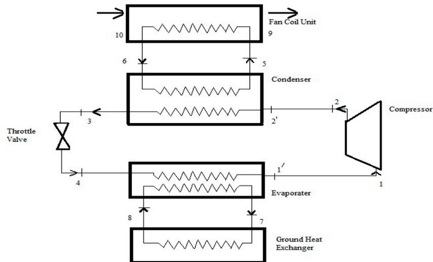
**Figure 5.** Schematic diagram of air conditioning system for summer operations.
