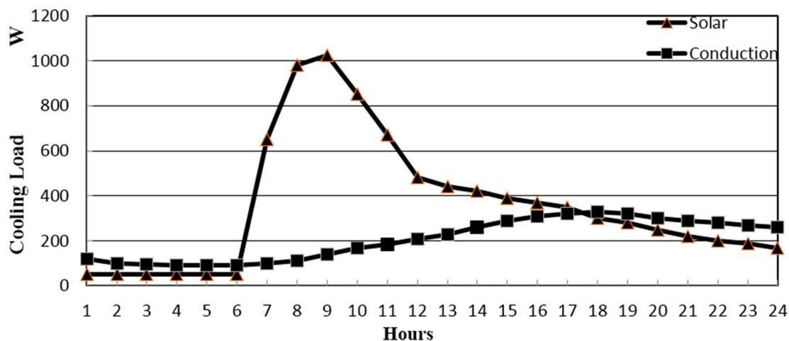
Figure 8. Hourly cooling load for fenestration.
