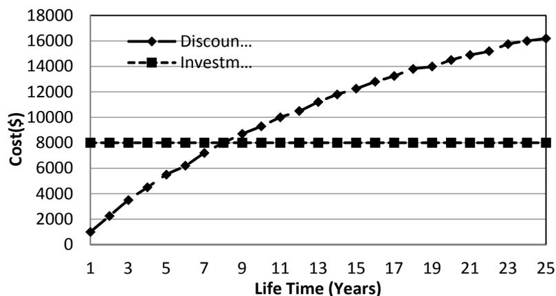
**Figure 17.** Discounted payback period of the geothermal heat pump system.
