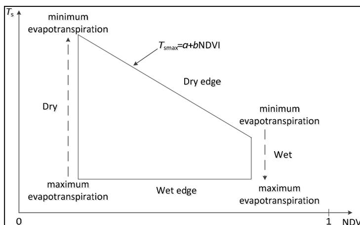
**Figure 4.** Definition of the TVDI. The TVDI for a given NDVI is estimated using  $T_s$ ,  $T_{smin}$  and  $T_{smax}$  (see Equation (2)).
