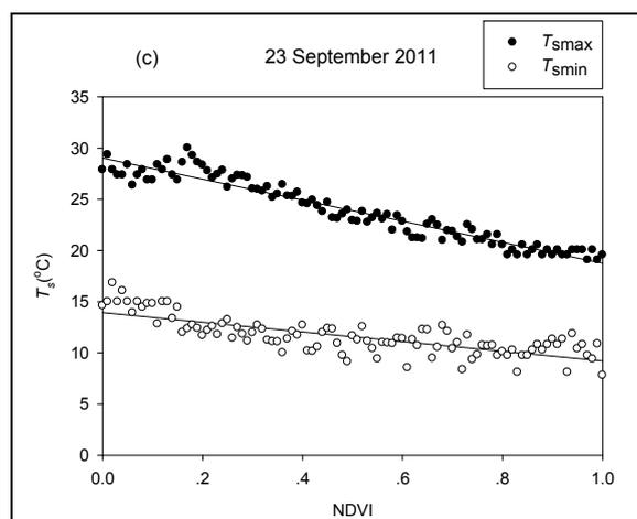
**Figure 5.** Plots of NDVI (x-axis) and surface temperature- $T_s$  (y-axis) in the study. The maximum  $T_s$  and minimum  $T_s$  are extracted for small intervals (0.01) of NDVI.
