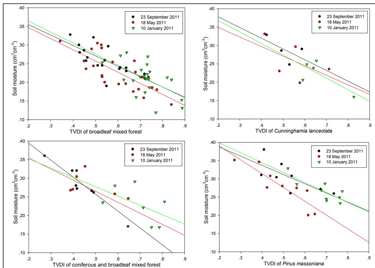
**Figure 7.** Comparison of the TVDI with the observation points of *in situ* soil moisture measurements for each land cover on 10 January 2011, 18 May 2011 and 23 September 2011.
