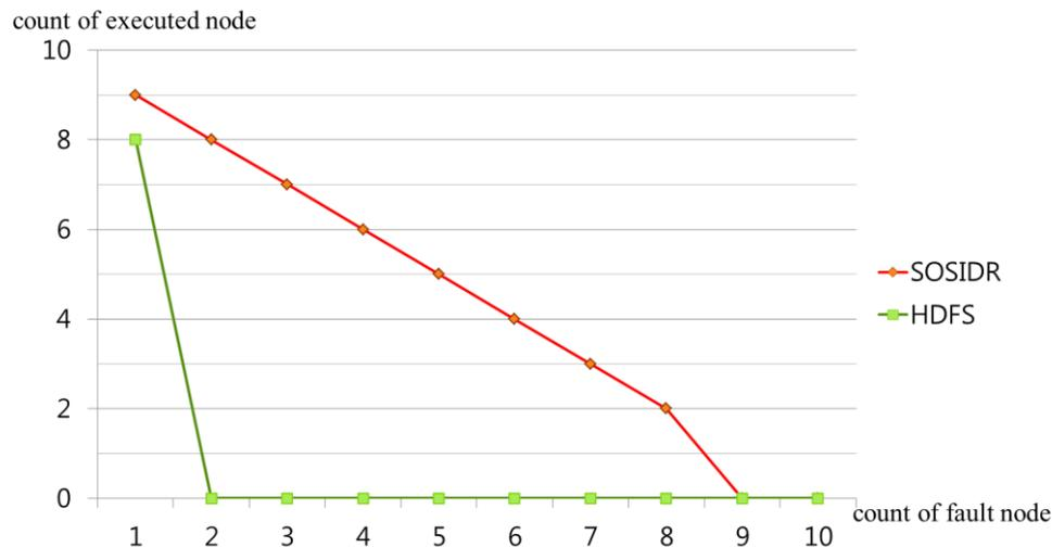
**Figure 6.** Comparison of the states of desktop operation that occur when a master node fault has occurred.
