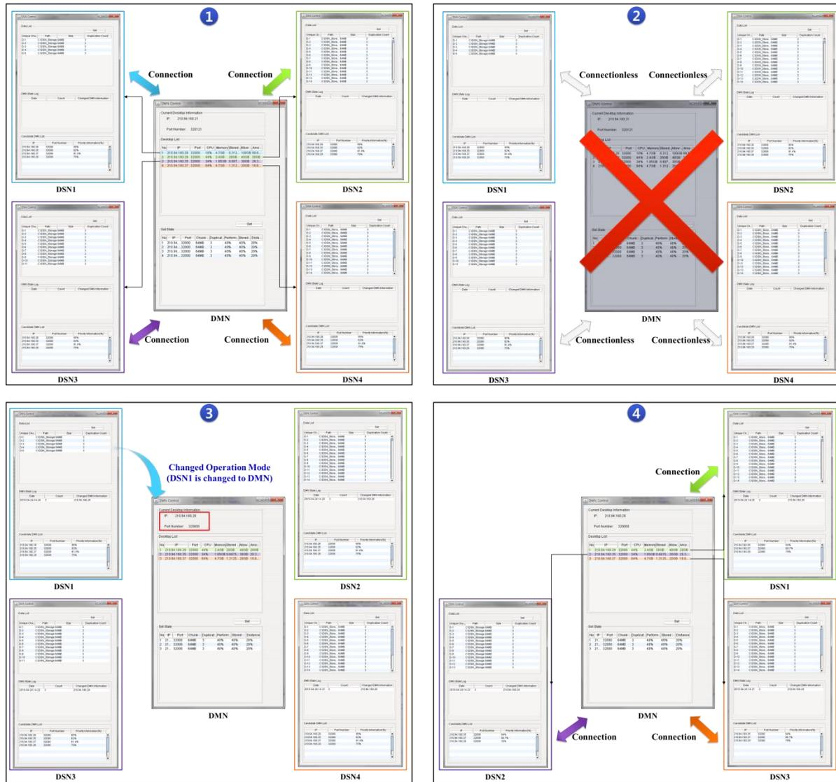
Figure 5. Response process for DMN faults in SOSIDR.
