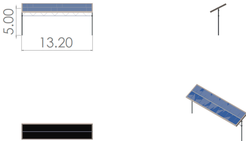
Figure 1. Basic layout of a single solar PV shed on an agrivoltaic farm. Source: The result of the authors' calculations using SOLIDWORKS® 2022 and Table 1 (2024) data.
