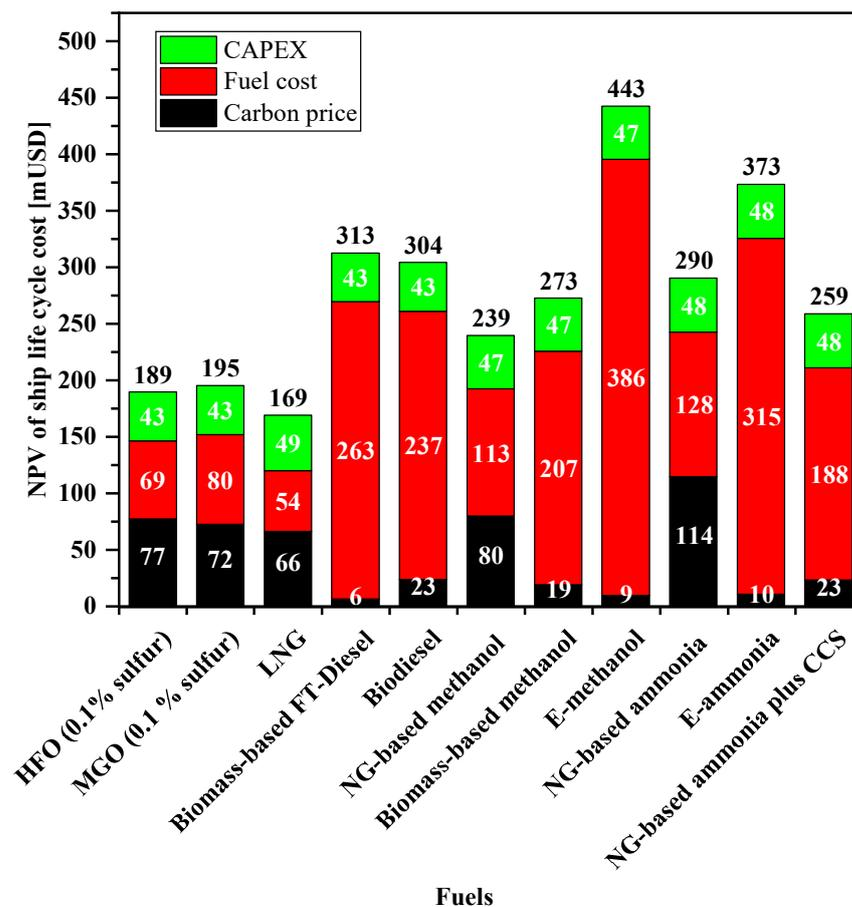
Figure 13. NPVs of ship life cycle costs including carbon price.
