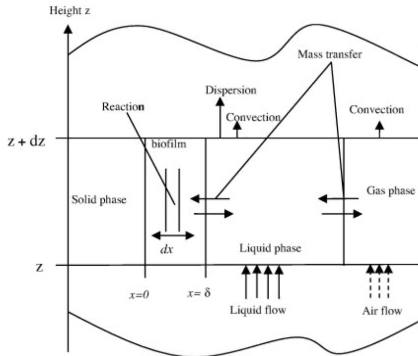
**Figure 2.** The mechanisms and the corresponding phases involved in a fluidized bed biofilm reactor [58]. Reprinted with permission from reference [58], License Number 56558201823.69.
