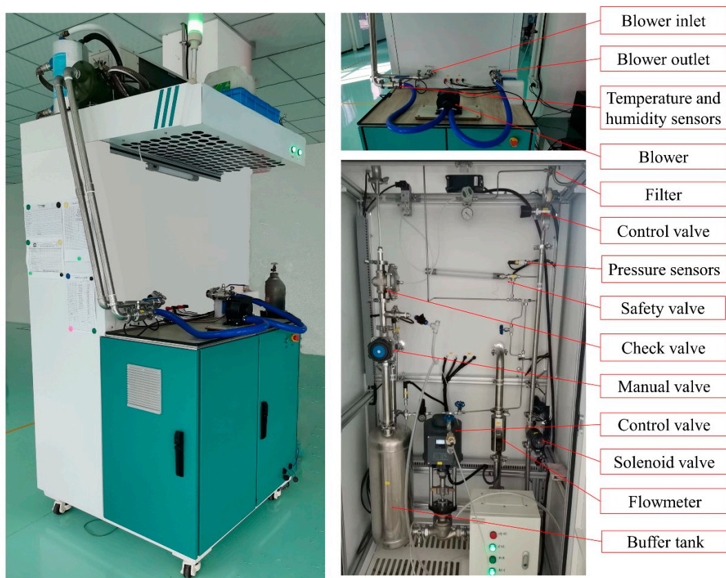
Figure 5. Test rig for the regenerative blower.
