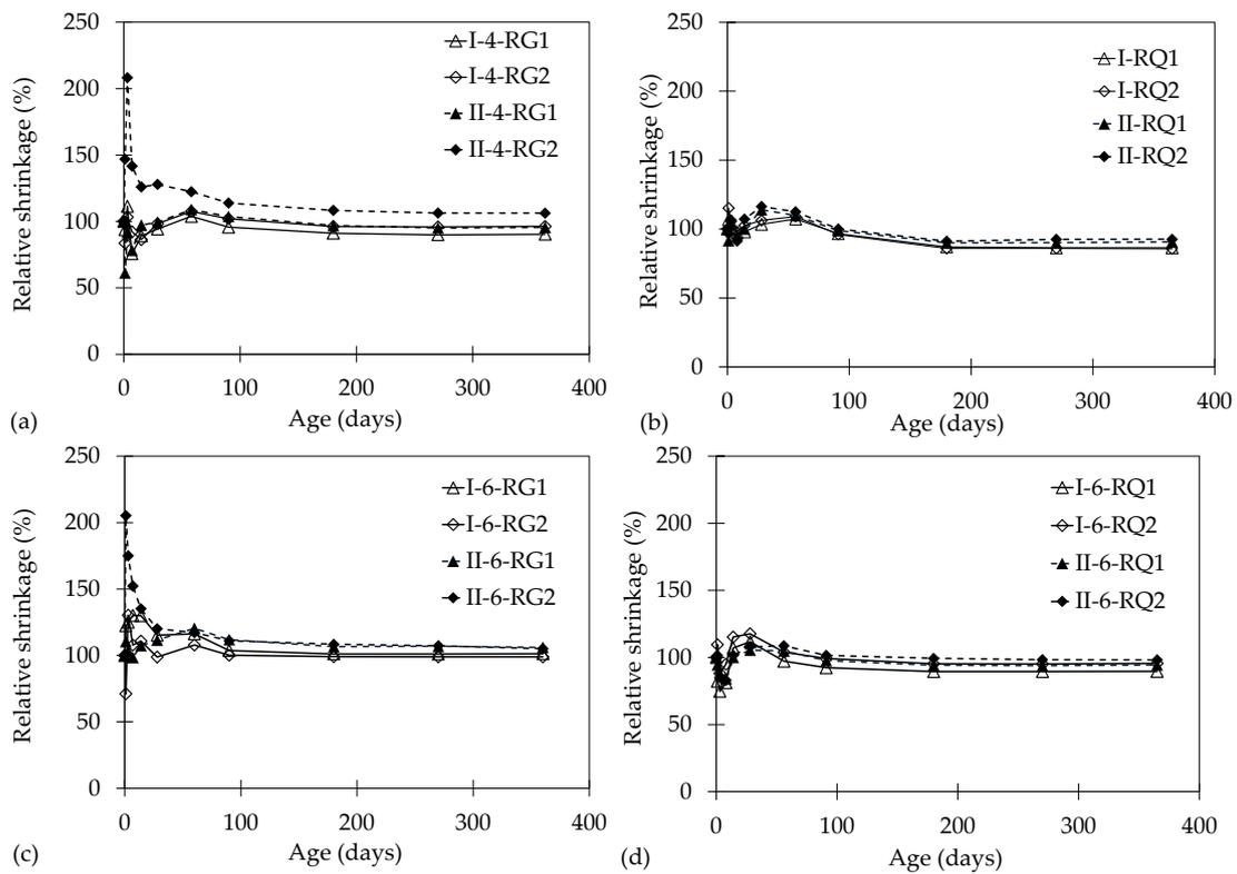
**Figure 6.** Drying shrinkage of recycled concretes relative to the reference concrete. (a) Granite recycled concretes,  $w/c = 0.40$ . (b) Quartzite recycled concretes,  $w/c = 0.40$ . (c) Granite recycled concretes,  $w/c = 0.55$ . (d) Quartzite recycled concretes,  $w/c = 0.55$ .
