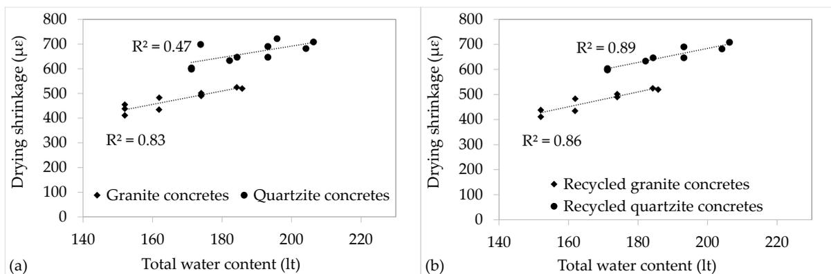
**Figure 7.** Relationship between drying shrinkage and total water content of reference and recycled concretes. (a) Reference and recycled concretes. (b) Only recycled concretes.
