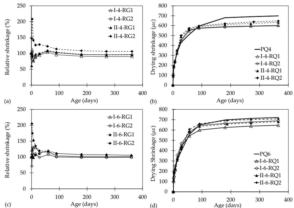
Figure 5. Drying shrinkage development over time. (a) Granite concretes, w/c = 0.40. (b) Quartzite concretes, w/c = 0.40. (c) Granite concretes, w/c = 0.55. (d) Quartzite concretes, w/c = 0.55.
