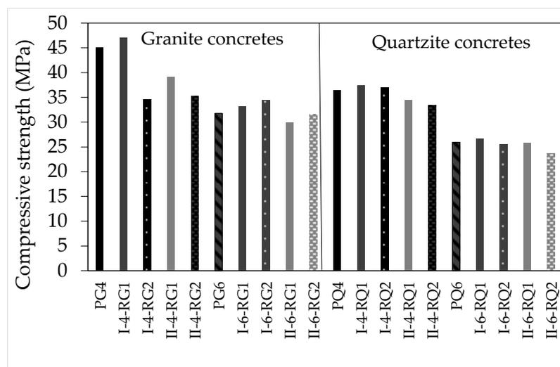
**Figure 1.** Compressive strength of concretes.
