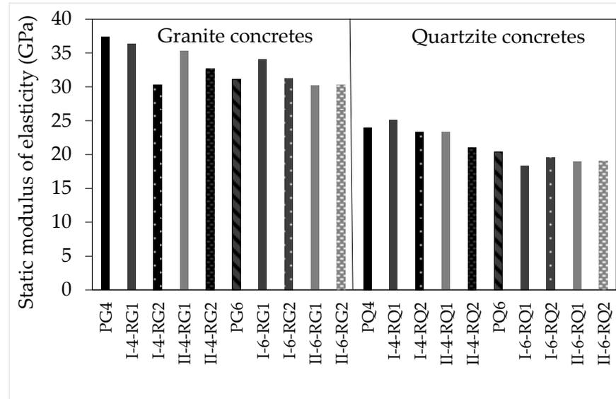
Figure 4. Static modulus of elasticity of concretes.
