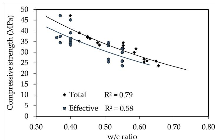
**Figure 2.** Relationship between compressive strength and total and effective w/c ratios.
