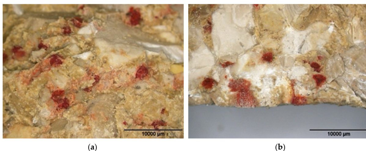
Figure 12. Mastic pigmentation due to type B capsules in loaded specimens: (a) AC 14; (b) SMA 11.
