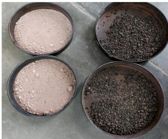
**Figure 1.** Stone aggregates: silt (left) and gravel (right).
