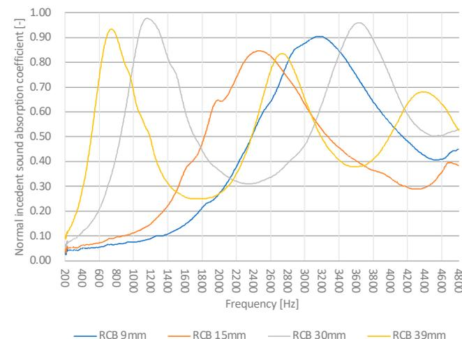
Figure 5. Comparison of measurement results of the RCBs’ sound absorption coefficients by thickness (200–4800 Hz).
