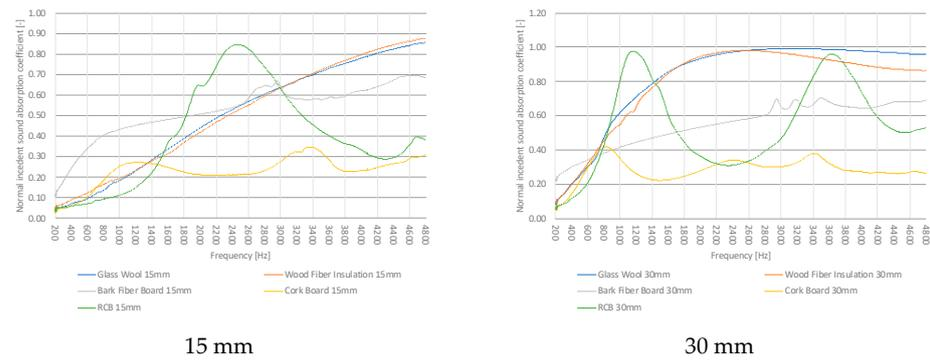
Figure 9. Comparison of measurement results of the sound absorption coefficients of porous materials (200–4800 Hz).
