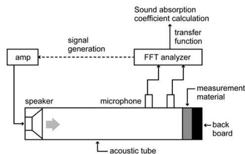
**Figure 2.** Measurement system for normal incidence sound absorption coefficient using an acoustic tube.
