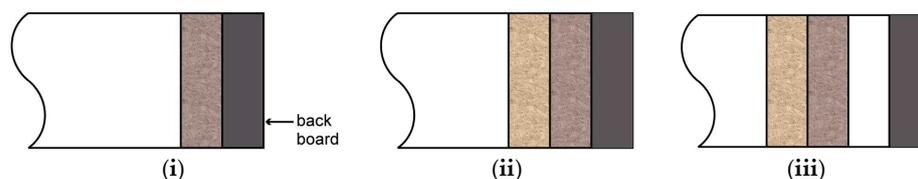
**Figure 3.** Installation conditions of the specimen. (i) Single material, (ii) RCB + porous material, (iii) RCB + porous material + back-air layer.
