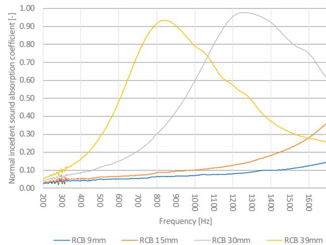
**Figure 6.** Comparison of measurement results of the RCBs' sound absorption coefficients by thickness (200–1600 Hz).
