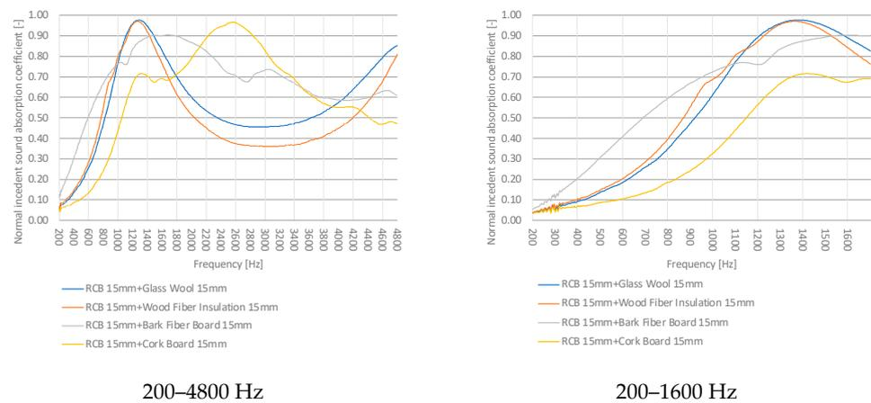
**Figure 12.** Comparison of measurement results of the sound absorption coefficient of multi-layered porous materials (15 + 15 mm).
