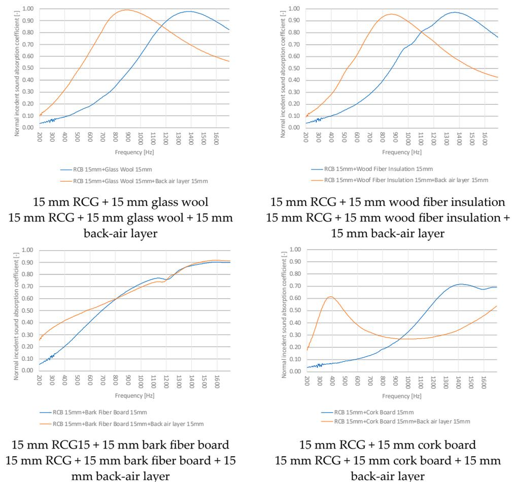
**Figure 16.** Comparison of measurement results of the sound absorption coefficients of multi-layered porous materials (15 + 15 mm) and multi-layered porous materials (15 + 15 mm) with back-air layer (15 mm).
