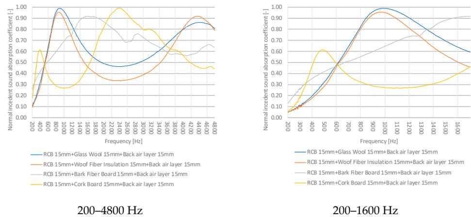
**Figure 15.** Comparison of measurement results of the sound absorption coefficients of multi-layered porous materials (15 + 15 mm) + back air layer (15 mm).
