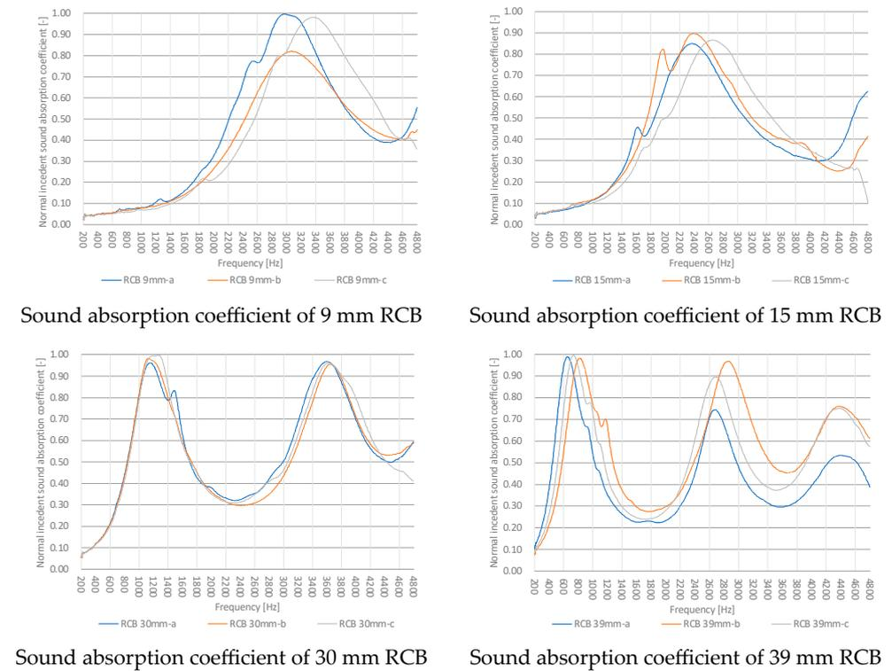
Figure 4. Measurement results of the RCBs’ sound absorption coefficients by thickness.
