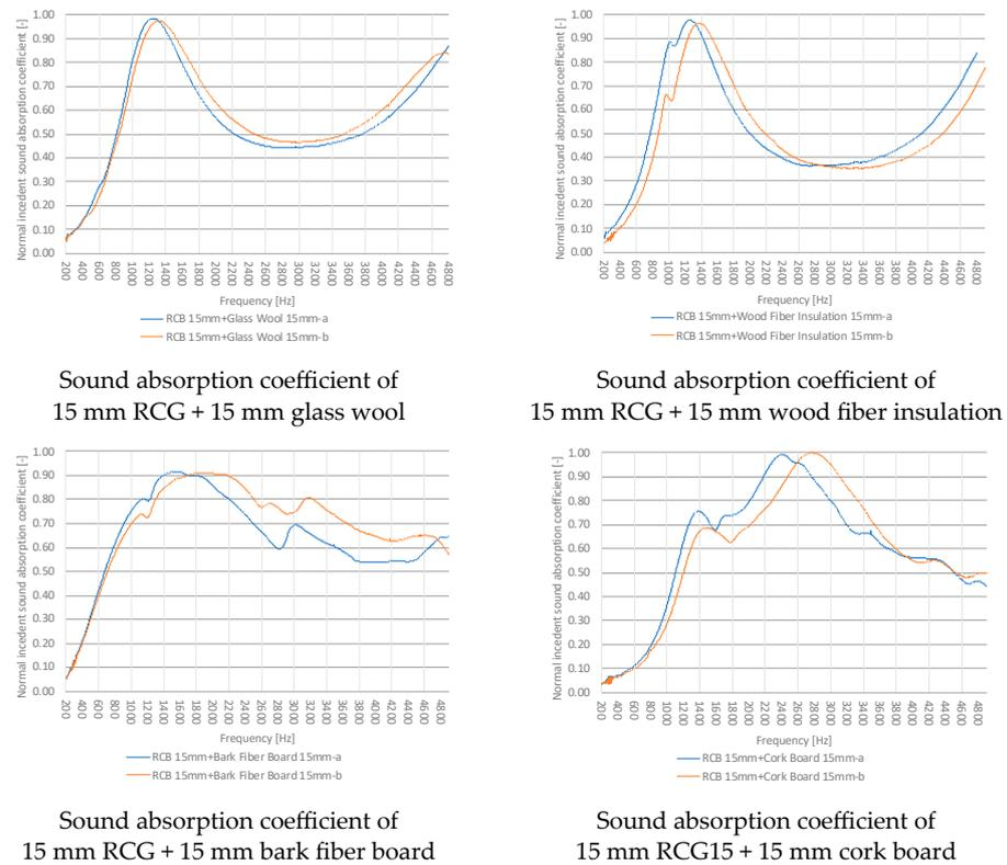
Figure 11. Measurement results of the sound absorption coefficient of multi-layered porous materials (15 + 15 mm).
