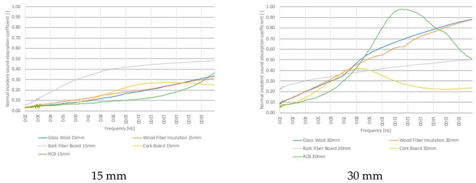
Figure 10. Comparison of measurement results of the sound absorption coefficients of porous materials (200–1600 Hz).
