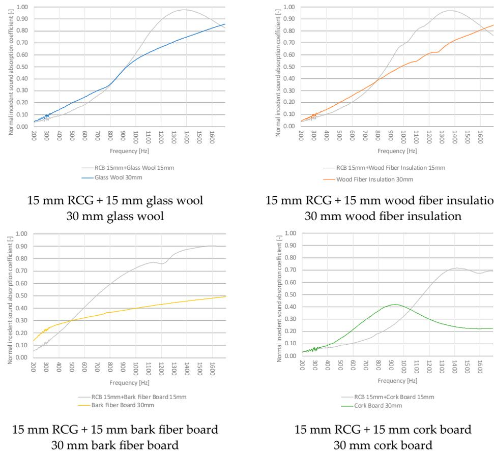
**Figure 13.** Comparison of measurement results of the sound absorption coefficients of multi-layered porous materials (15 + 15 mm) and porous material (30 mm).
