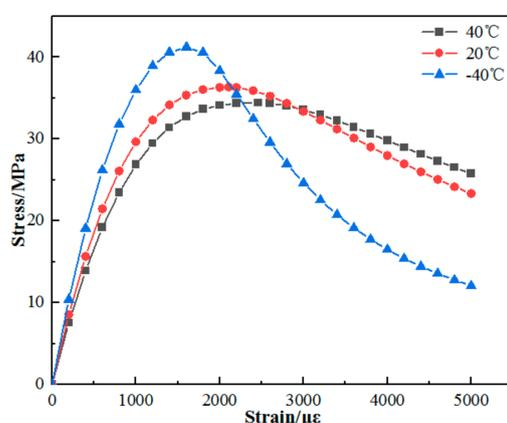
**Figure 5.** Theoretical stress-strain curves of concrete at different temperatures.
