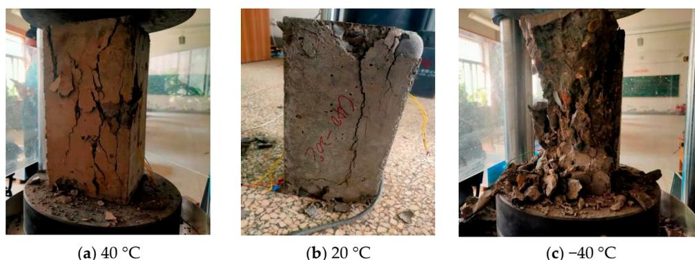
**Figure 3.** Concrete prism failure mechanisms at different temperatures.
