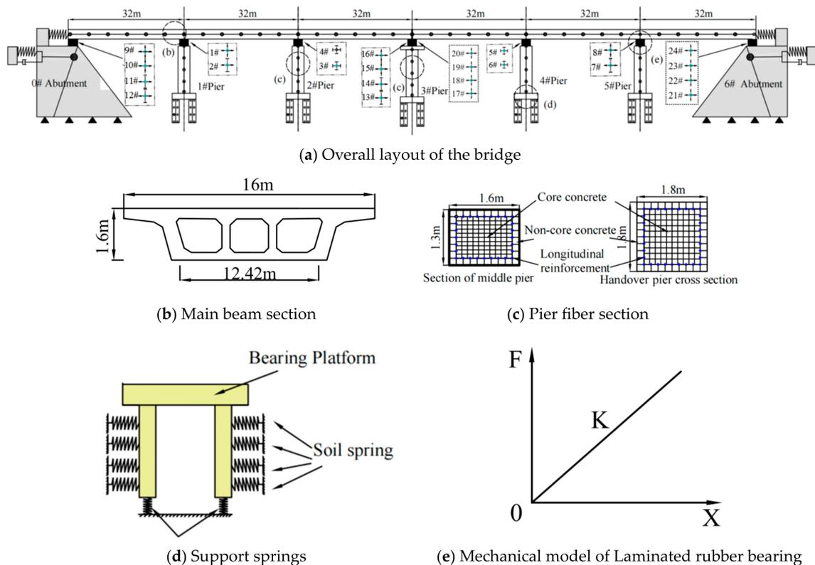
**Figure 1.** Finite element model of bridge.
