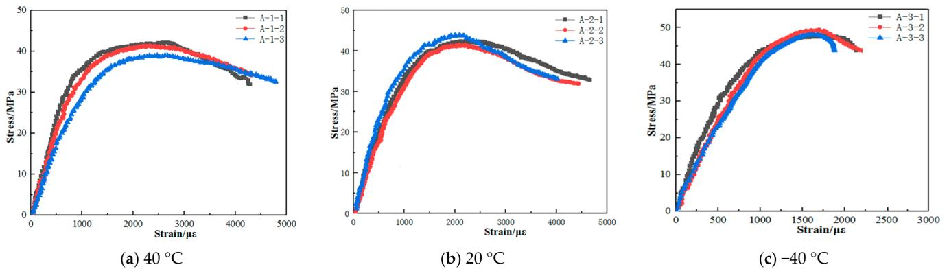
**Figure 4.** Concrete stress-strain curves under different temperatures.
