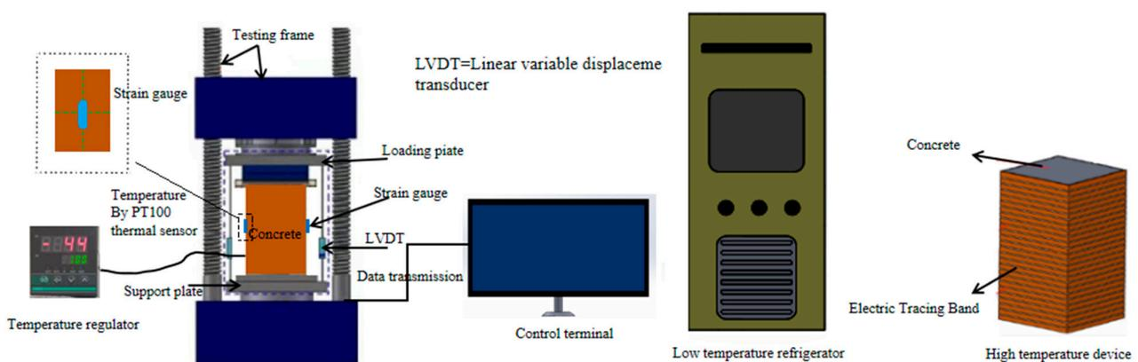
**Figure 2.** High and low temperature devices and loading equipment.
