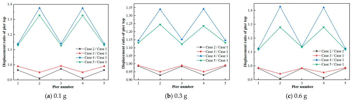
Figure 8. Displacement ratio of the pier tops of each case to case 1.
