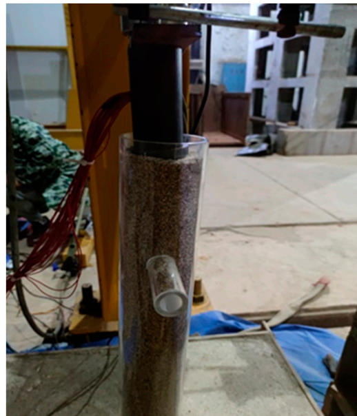
Figure 15. Instability of model pile (Simplified Model of a Plexiglas Tube).
