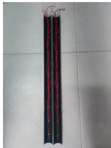
Figure 5. Model pile strain gauge pasting.
