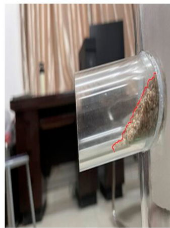
Figure 12. Sand heap shape-simulation diagram of No. 2 Karst cave after pipe pull out.
